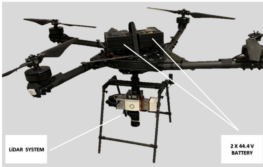
Figure 2. Freely Systems ALTA-X quadcopter with the attached RIEGL LiDAR payload. This UAS system boasts 4 motors generating 17,760 watts of max continuous power lending to a maximum gross takeoff weight of 34.9 kg and a total flight time configure as seen of roughly 10.75 minutes.
