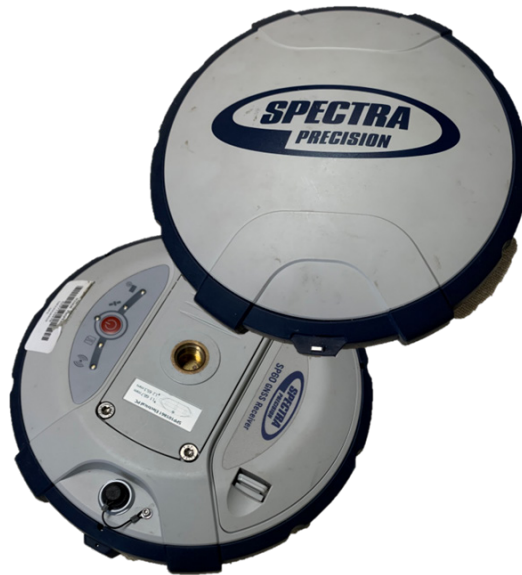
Figure 4. GPS puck used as a static base station. This puck was mounted on a tripod roughly 5 ft high in a position near the UAS launch site.
