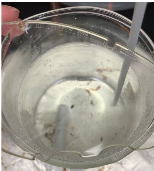
Figure 4. BPMPC copolymer applied and cured on WileyX lens, which had the factory antifog coating removed.
