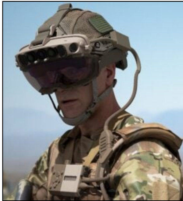
Figure 22. Fully Ruggedized and Militarized Version of Integrated Visual Augmentation System. Source: Freedberg (2022).
