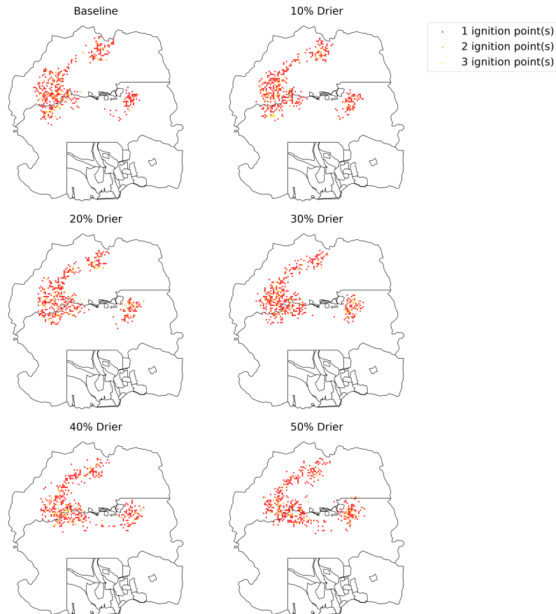
Figure 4.8. Ignition Points of Largest 10% of Fires at Hour 72. The invariance of these points under increasing dryness conditions suggests some areas are always at higher risk of producing large fires.
