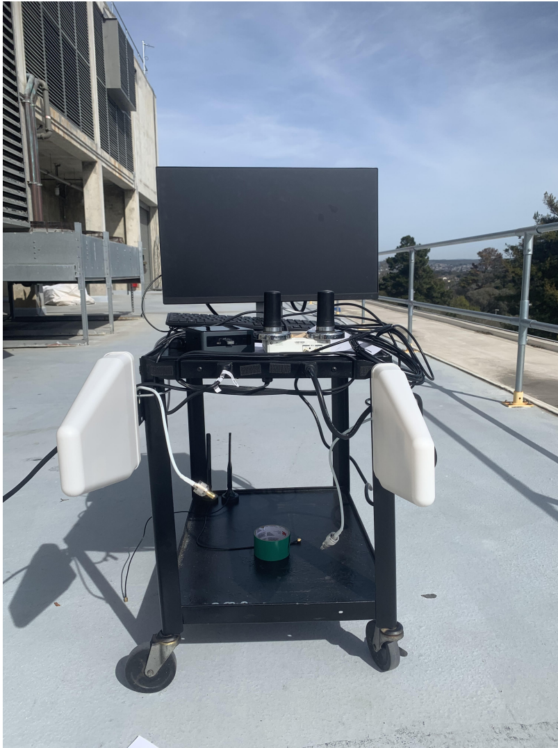
Figure 4.15. Physical testing setup showing the mounted directional antennas on a mobility cart, along with display, SDR, and NUC controller
