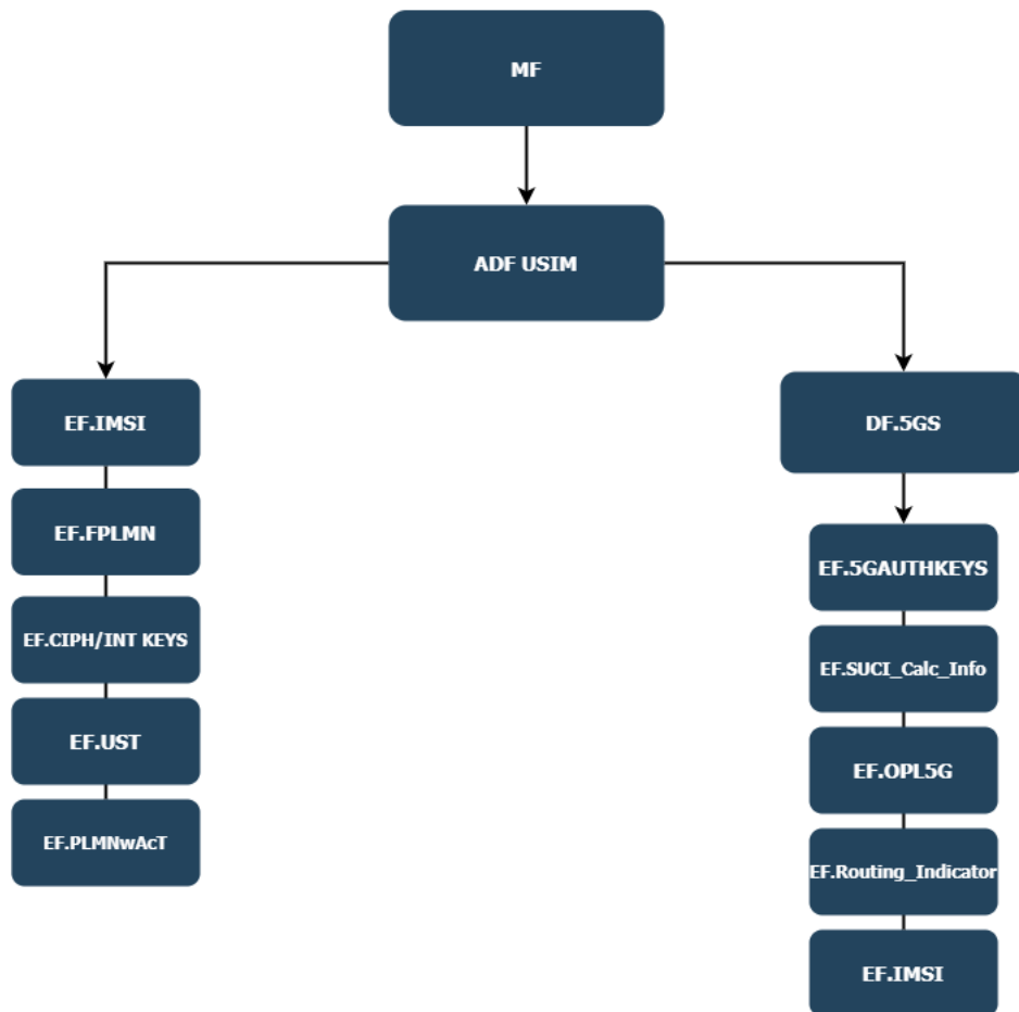
Figure 3.12. USIM file structure
