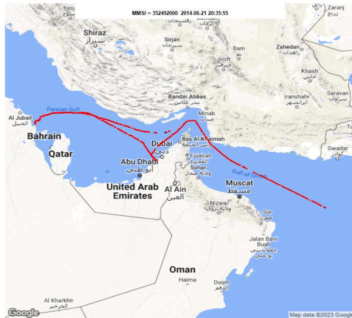
Figure 3.4. Example of a vessel transiting to multiple destinations in the Persian Gulf. Each AIS transmission for this vessel track is plotted as a small, red circle using the “leaflet” package in R. Source: Cheng et al. (2022).
