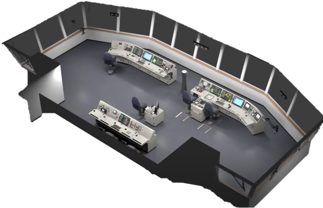
Figure 2. Bridge consoles that house IBS and IPMS workstations. Adapted from OSI Maritime Systems (n.d.).
