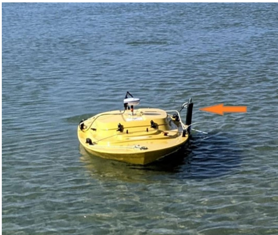
Figure 13. Aqua TROLL ® 600 sensor mounted to the Z-boat ® (orange arrow).
