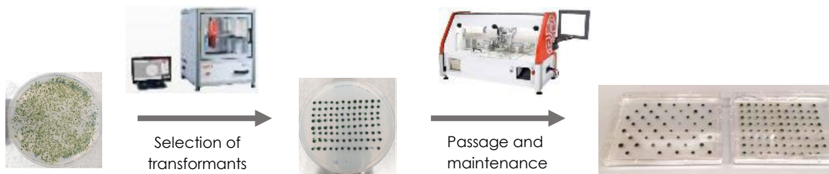
Figure 10. Automation-assisted screening of transformed Chlamydomonas . Positive transformants were selected using the Singer PIXL, which automates imaging, colony recognition, colony selection, and picking from culture plates. Transformants were continually passaged on culture media containing 10 mg/L zeocin using the Singer RoToR HDA pinning robot designed for rapid picking and re-plating of microorganism colonies. Photos: Singer Instruments.
