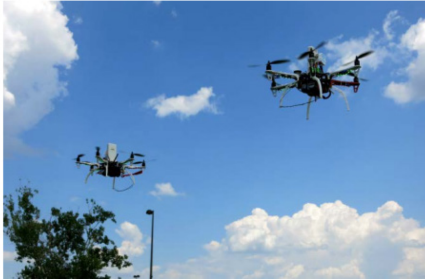
Figure 64. Drone deployment, outfitted with Wi-Fi and UHF radio communication payload. Source: NPSTC (2018)
