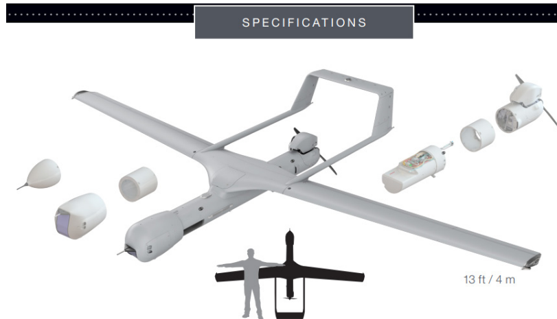
Figure 13. ScanEagle 3 small tactical UAS. Source: Insitu (2020).
