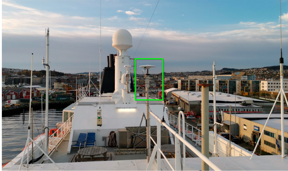
Figure 59. GNSS antenna mounted on board the Hurtigruten vessel sailing from Bergen to Kirkenes, Norway. Source: Susi, M. et al. (2021).
