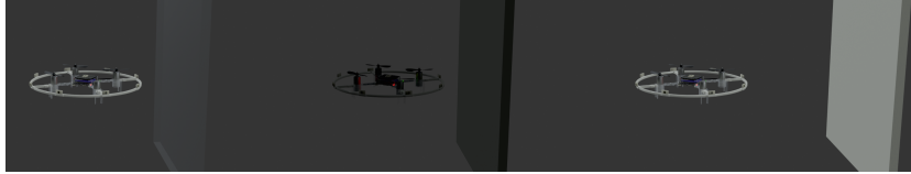
Figure 20: Representation of the three failure modes avoided by our sensor integration method, transparent, low-light conditions and distant surfaces. Note that the optical flow sensors are effective even in moderate light conditions, so the low light illustration is merely indicative.
