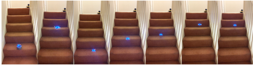
Figure 21: A sequence of still frames showing our drones capabilities when climbing a suburban staircase. The drone moves up the stairs consistently detecting the obstacles and avoiding them by invoking an override controller.
