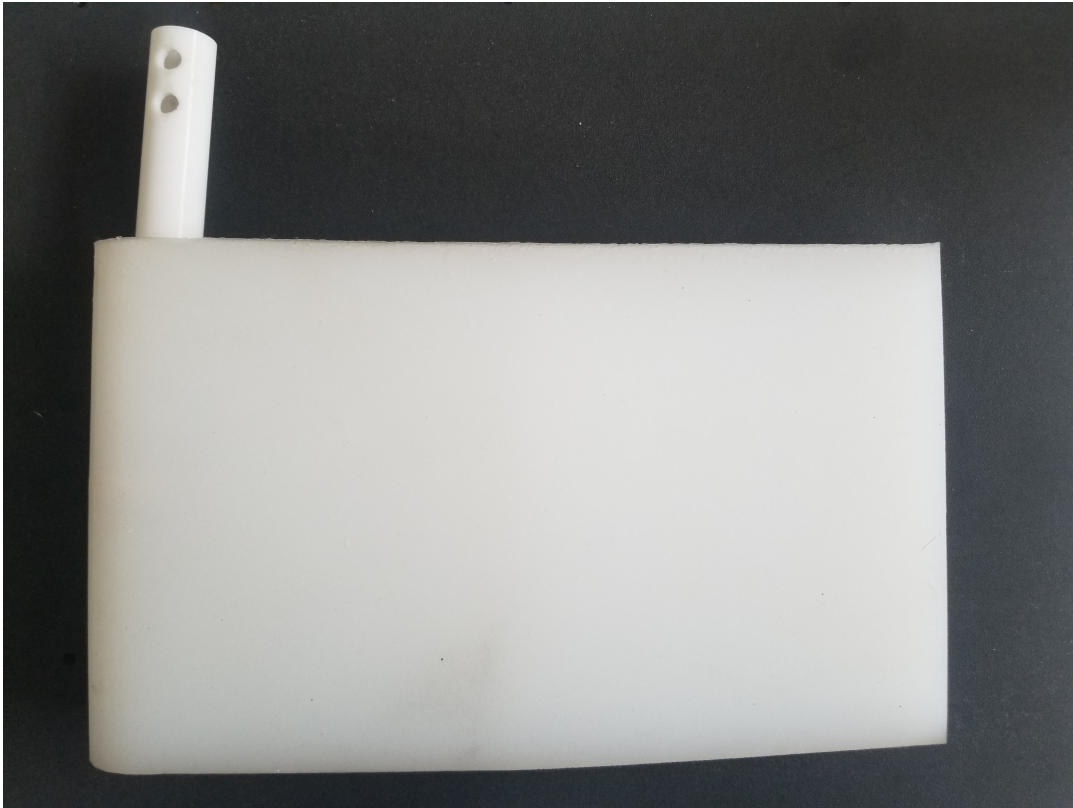
Figure 4.5. Cycle 3 flexible body with internal rotational adapter. Notice that the “L”-shaped portion of the adapter, as seen in Figure 4.1, has been removed.
