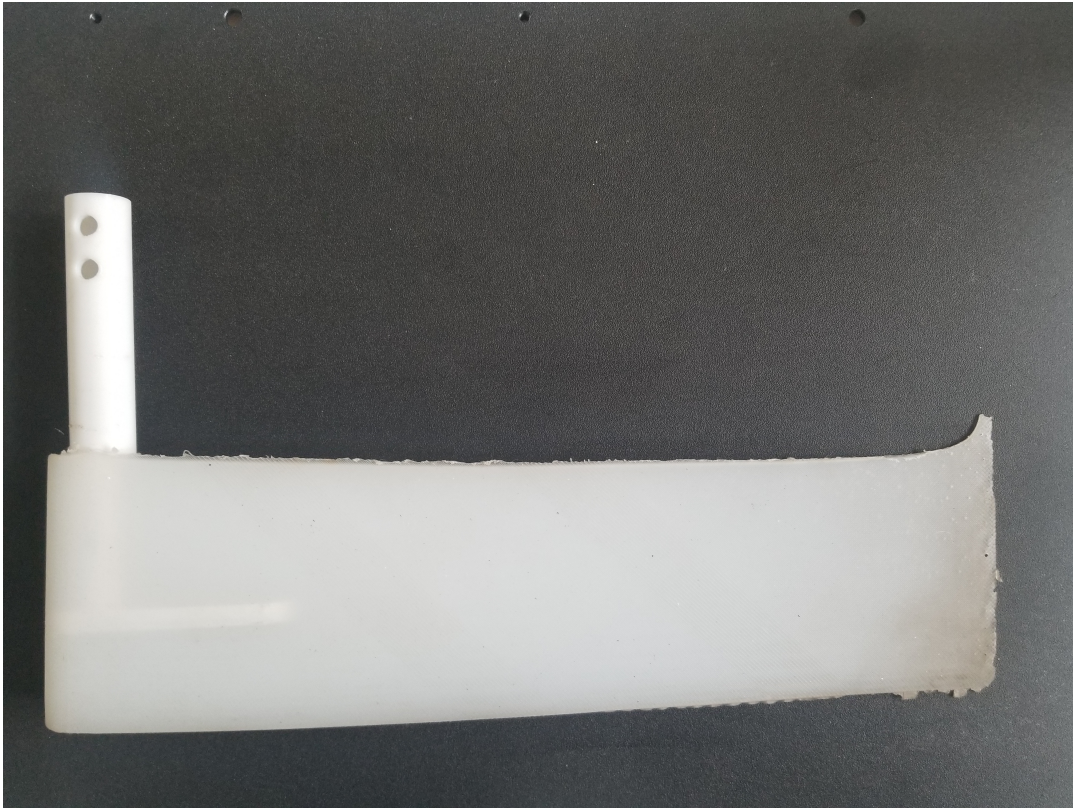
Figure 4.1. Cycle 1 pennant shaped flexible body with “L” shaped adapter.
