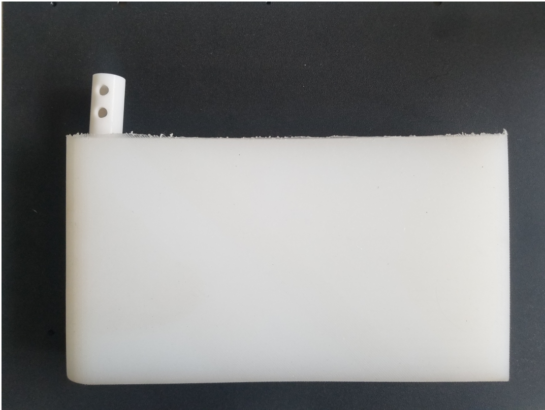
Figure 4.3. Cycle 2 4.445 cm (1.75 in) wide flexible body with “L” shaped adapter.
