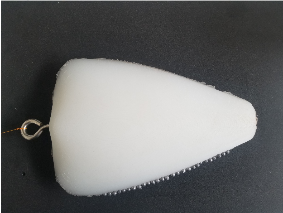
Figure 4.11. Cycle 5 free floating body with eyebolt and lead weights attached
