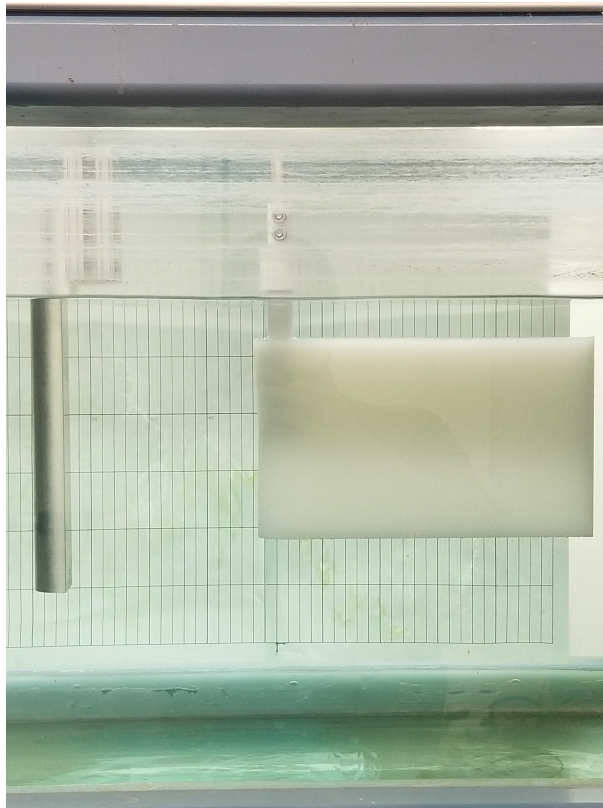
Figure 4.8. Updated external rotational insert design that fixed the previous cant problem.
