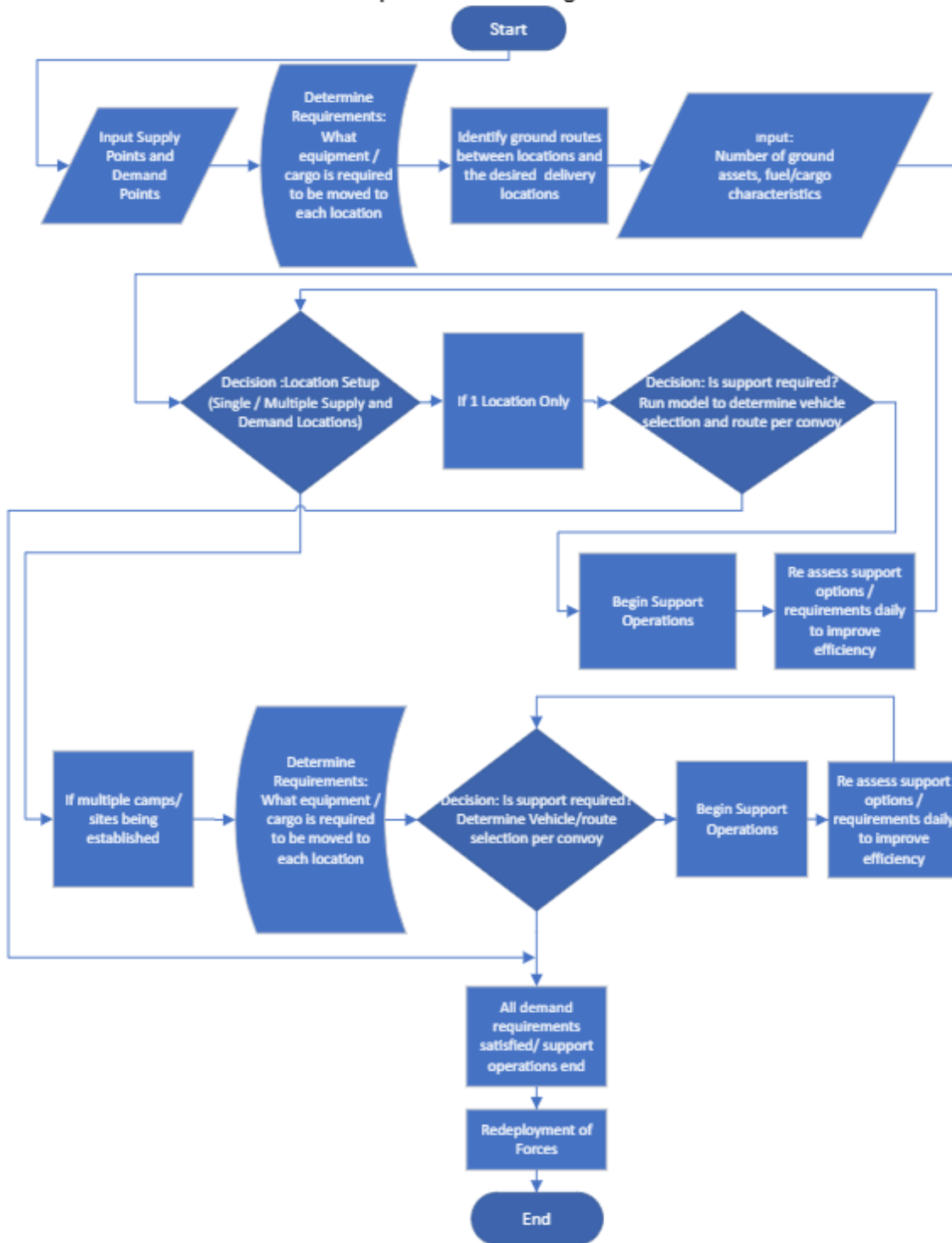
Figure 7. Ground Transportation Planning Process Flowchart.
