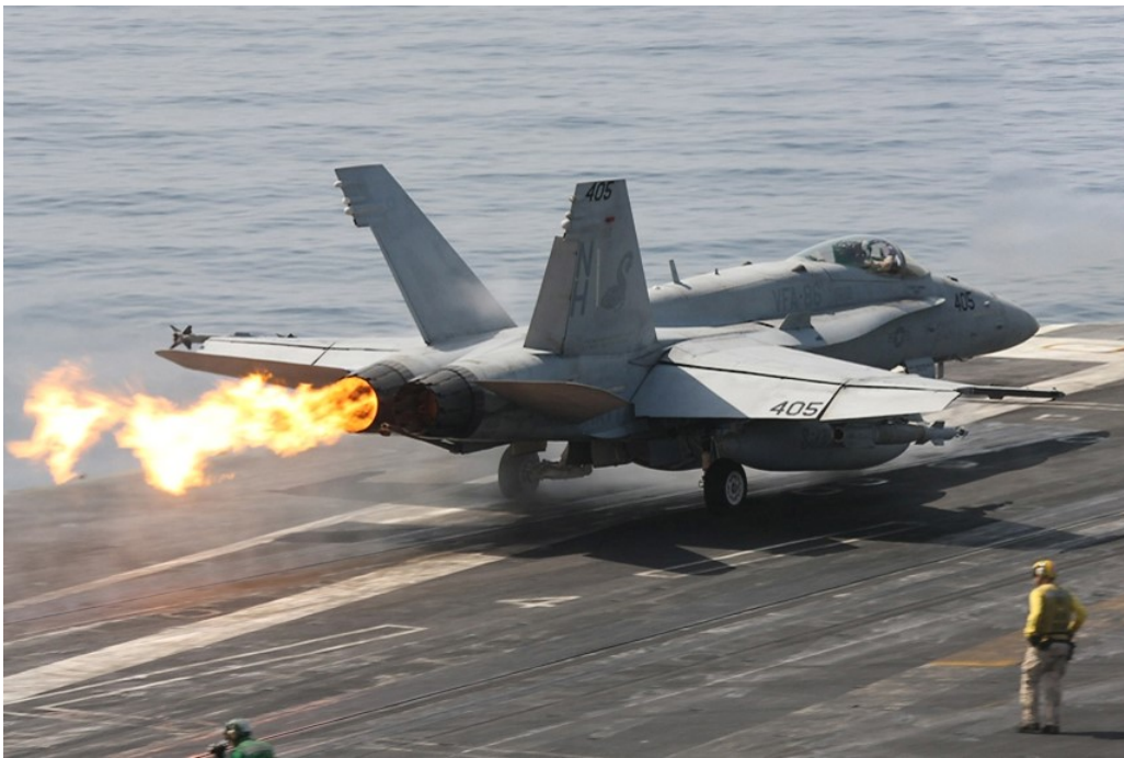
Figure 1.1. F/A-18C Suffers Compressor Stall During Carrier Takeoff. Source: [1]
