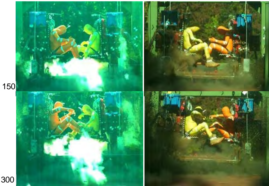
Figure D-1. Male (CORALS) shot 1 – Crew 1: 50 th percentile male, orange; Crew 2: 50 th percentile male, yellow
