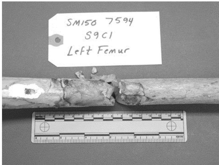
Figure E-132. Fracture of the left femur of S9C1 (anterior view, right is proximal)
