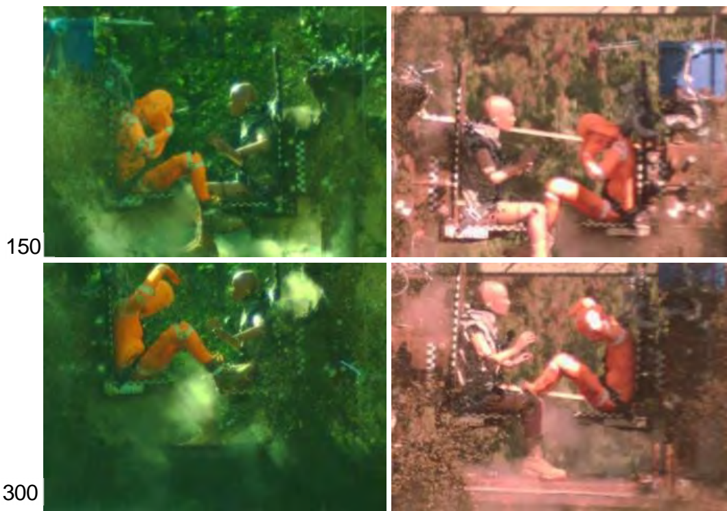
Figure D-6. Female shot 4 – Crew 1: 5 th percentile female, orange; Crew 2: Hybrid III 5 th percentile female ATD
