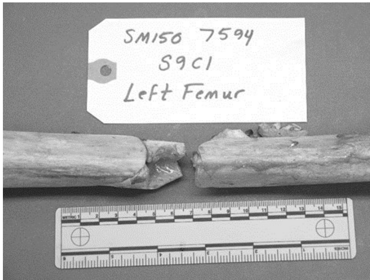
Figure E-134. Fracture of the left femur of S9C1 (posterior view, right is proximal)
