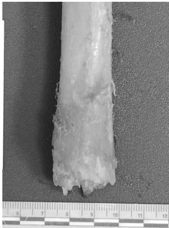
Figure E-46. Compression fracture of the left distal tibia of S5C1 (anterior view)
