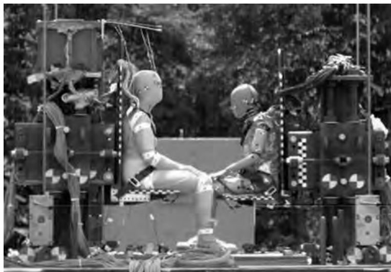
Figure 12. PMHS (left) and Hybrid III 5 th percentile female ATD (right) positioned on the ALF
