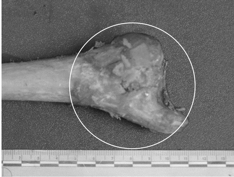
Figure E-58. Compression fracture of the left distal tibia of S5C2 (anterior view)
