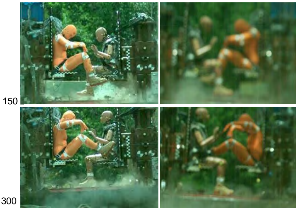
Figure D-4. Female shot 2 – Crew 1: 75 th percentile female, orange; Crew 2: Hybrid III 5 th percentile female anthropomorphic test device (ATD)
