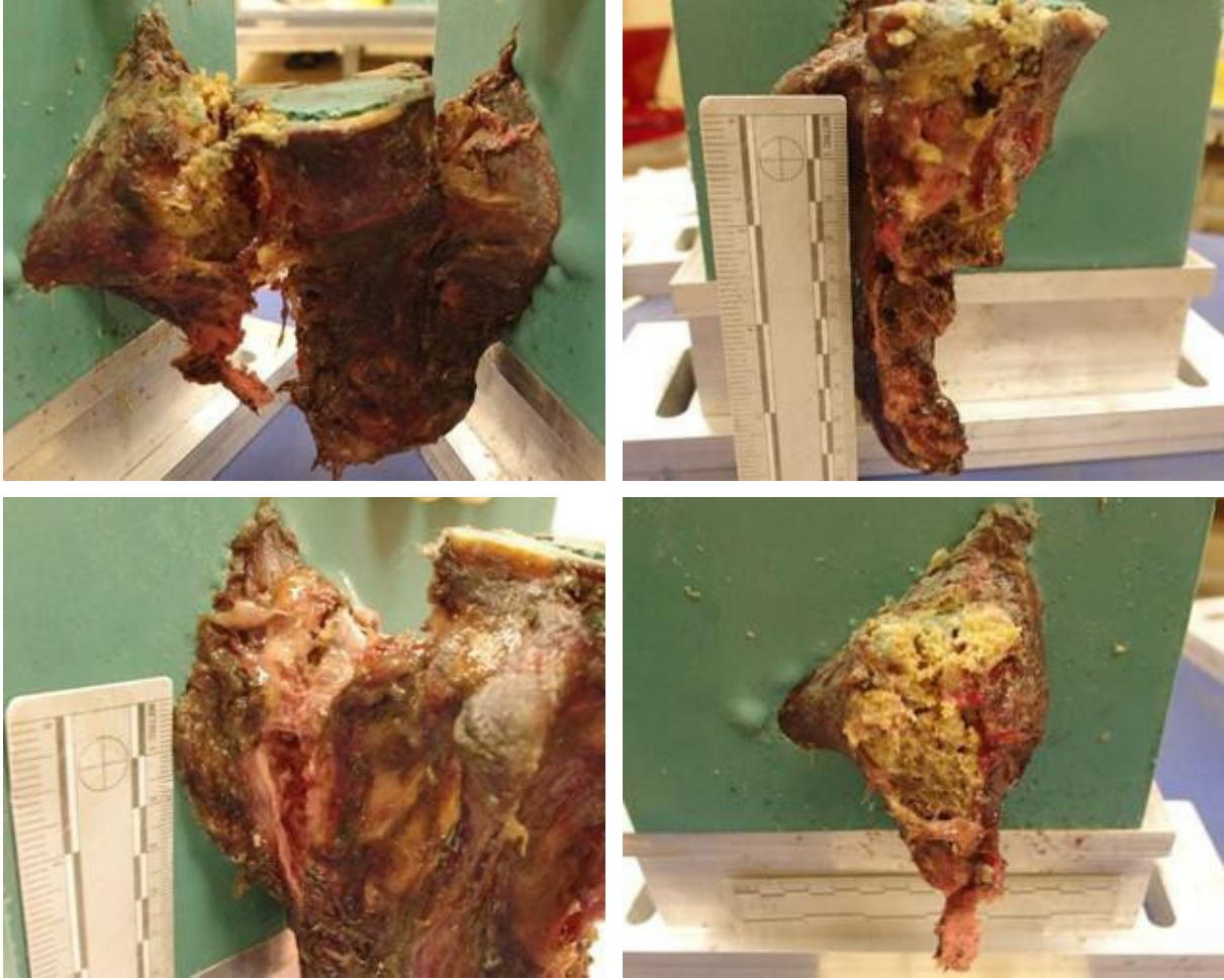
Figure E-13. Sacrum/pelvis damage for PMHSL7034: Pelvic perspective (top left), right sacral alae (top right), left sacral alae (bottom left), and right costal elements (bottom right)
