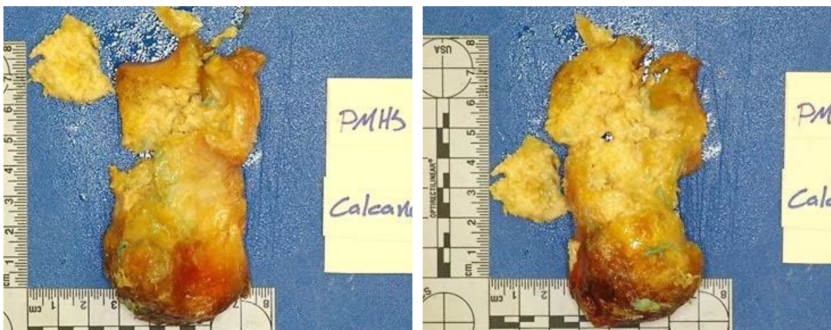
Figure B-13. Fracture of the right calcaneus plantar view (left) and sagittal view (right) of PMHS7607
