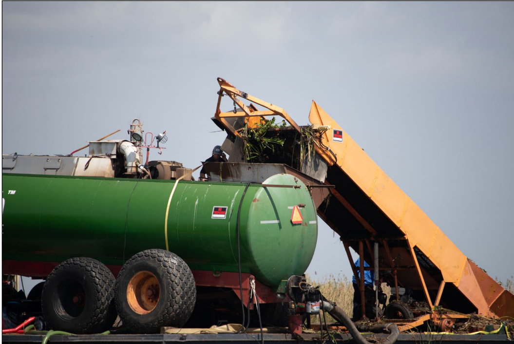
Figure 3. Water hyacinth plants being transferred from the elevator into the macerator press (juicer).
