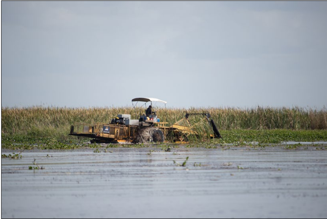
Figure 1. Aquatic-plant harvester collecting water hyacinth at the study site in Lake Okeechobee, Florida.
