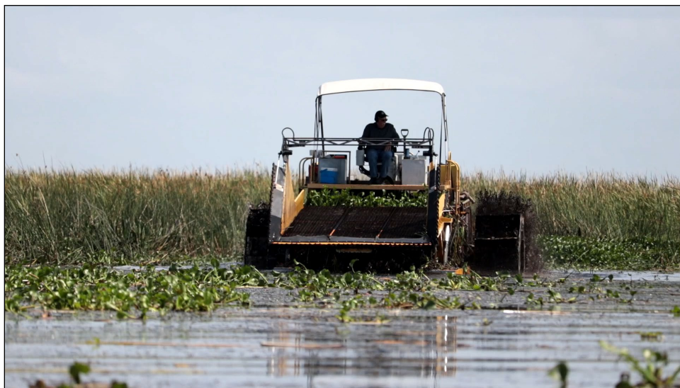
Figure 6. Aquatic-plant harvester operating in shallow water.
