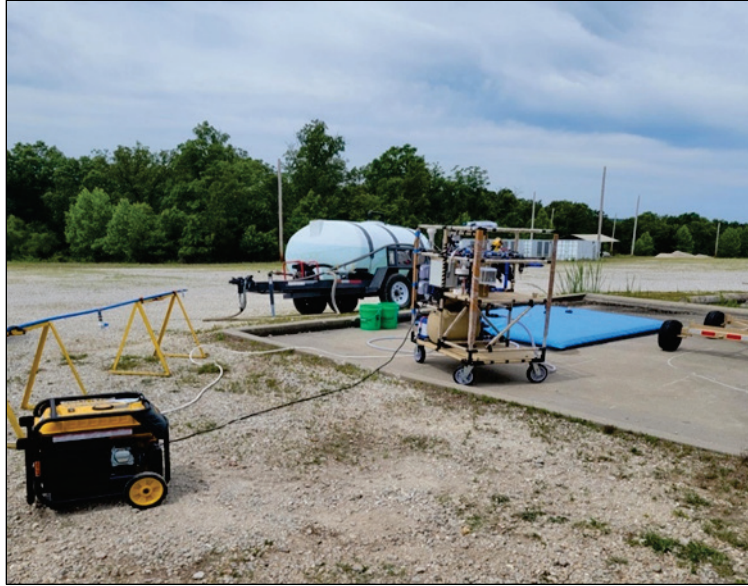
Figure 1. The ruggedized Water on Wheels (WOW) mobile emergency water treatment system, now called the Deployable Resilient Installation water Purification and treatment System (DRIPS) unit, set up for the user jury at Fort Leonard Wood (FLW) in June 2023.
