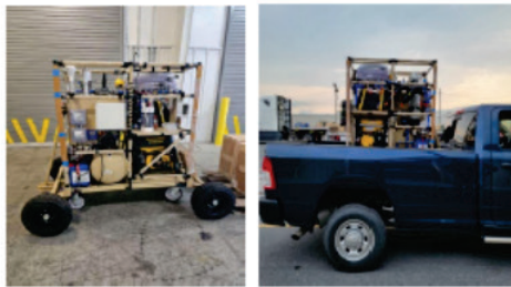
Figure 2: DRIPS mobile emergency water treatment system cart Organic Industrial Base 2023.
