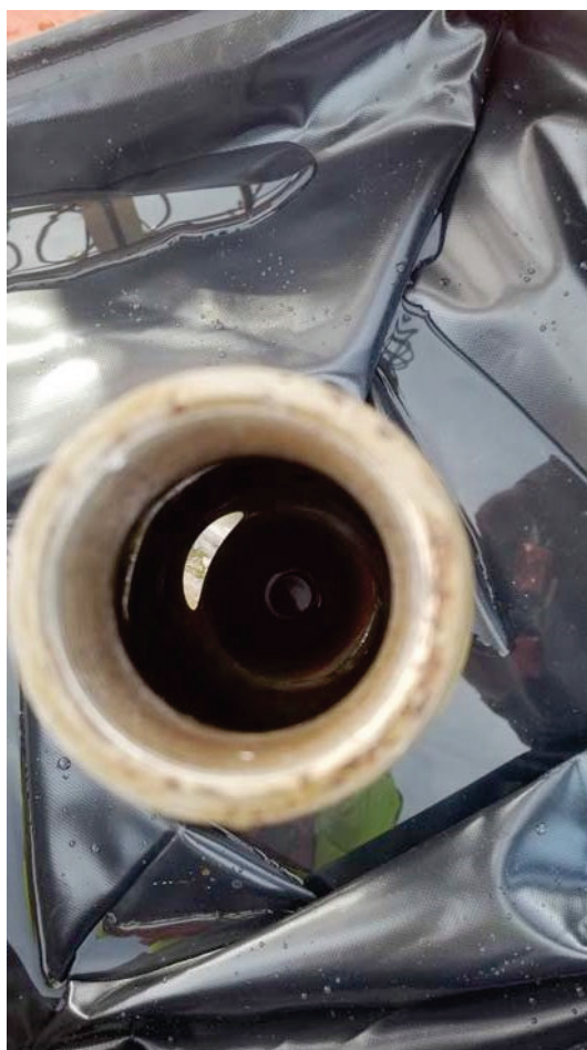
(b) Item 2 after processing; nose plug is removed to see that the base is completely clean
