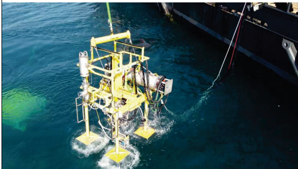
(b) Deployment of the Underwater Cut and Capture System with the ROV nearby
