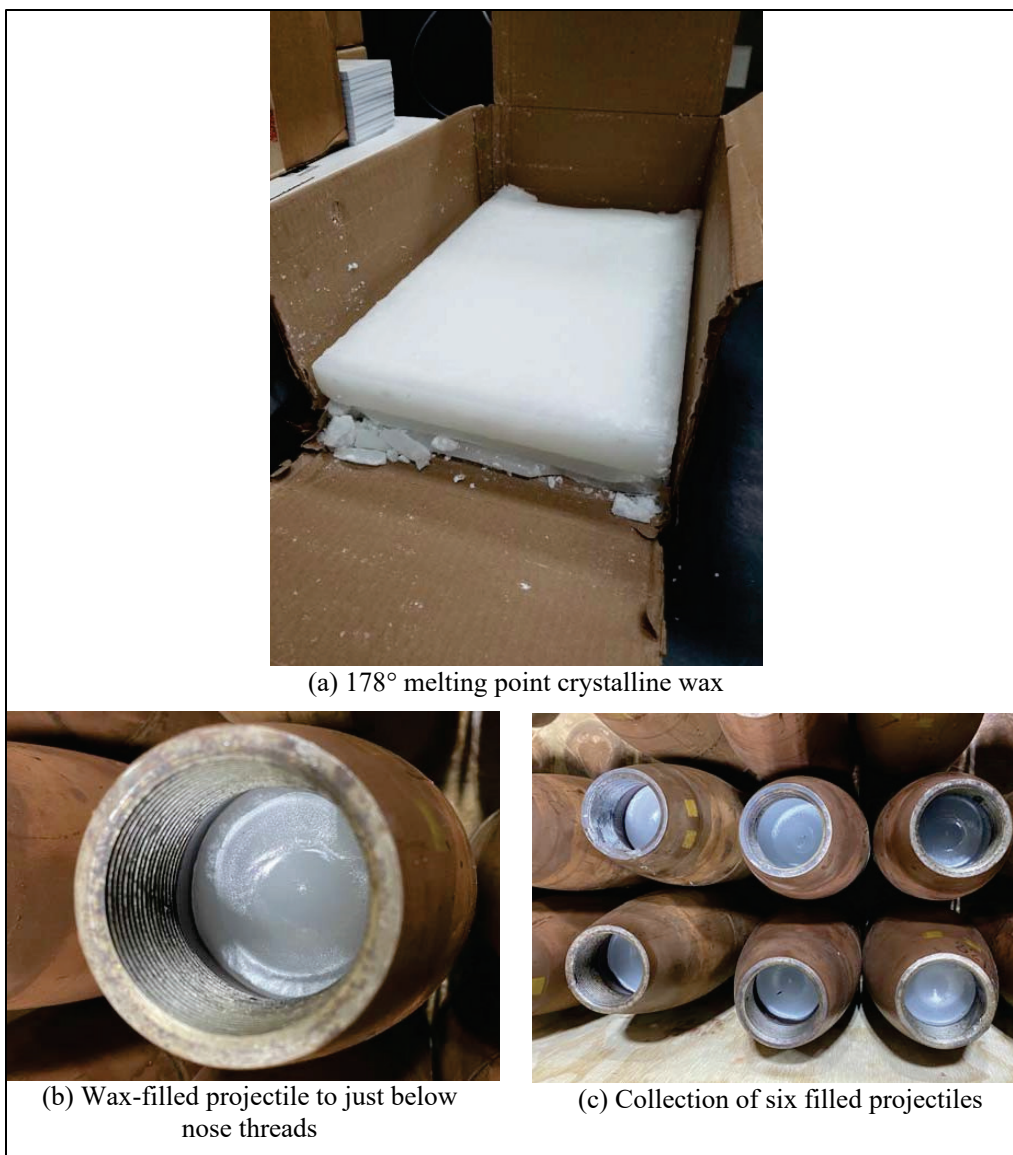
Figure 11. Army 105 mm HE M1 projectile bodies ( bottom ) filled with 178°F melting point microcrystalline wax ( top ).
