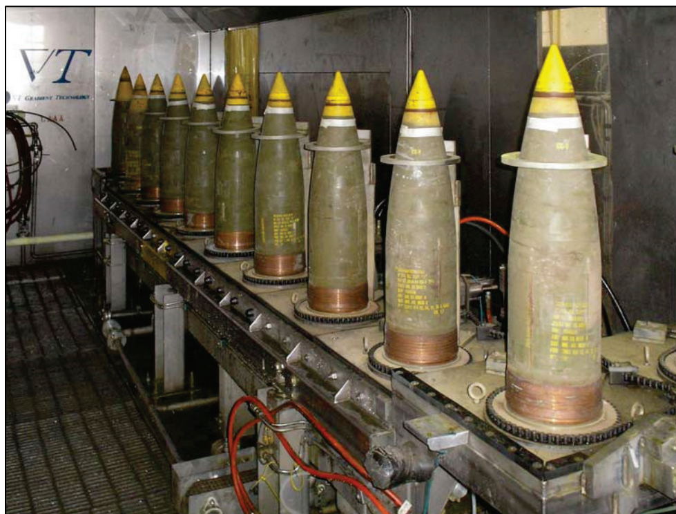
Figure 3. Automated abrasive waterjet (AWJ) cutting and washout system processing 8 in./55 cal high capacity (HC) rounds.
