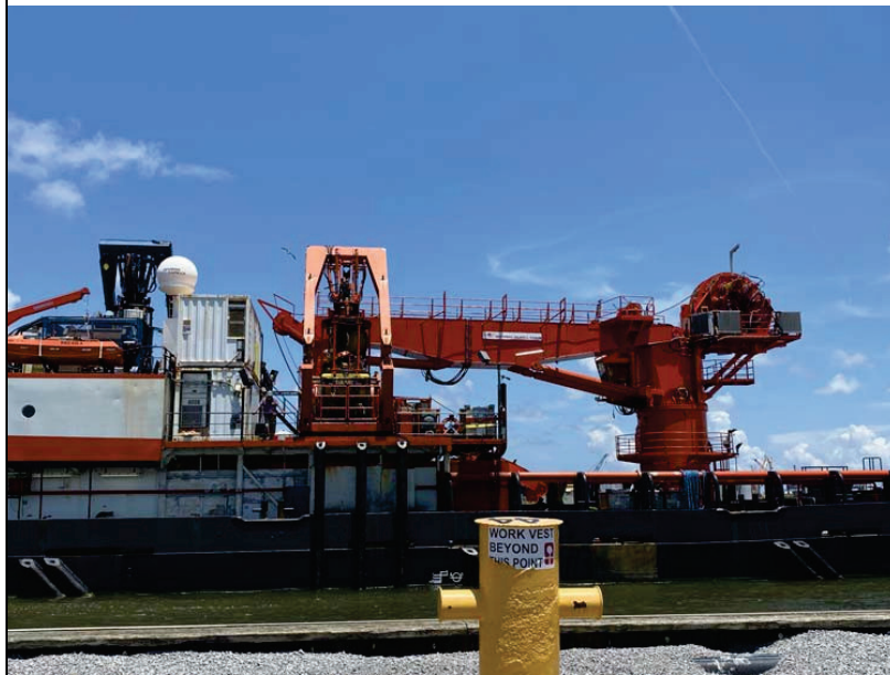
(b) View of the 200 ton crane used to deploy the Underwater Cut and Capture System
