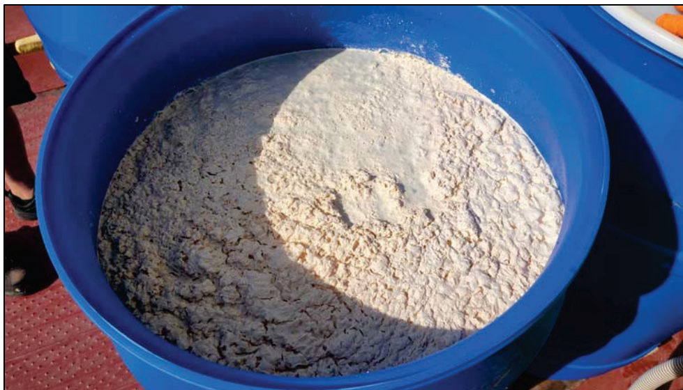
(a) TNT and water mixture collected after processing a TNT-filled 105 mm projectile
