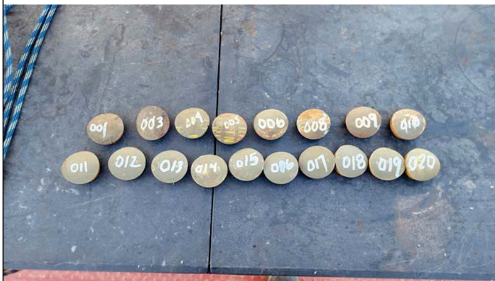
(b) Cut plugs from some of the processed projectiles
