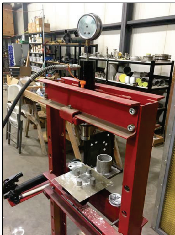
Figure 8. Hydraulic press for pressing the inert fill into the target items.
