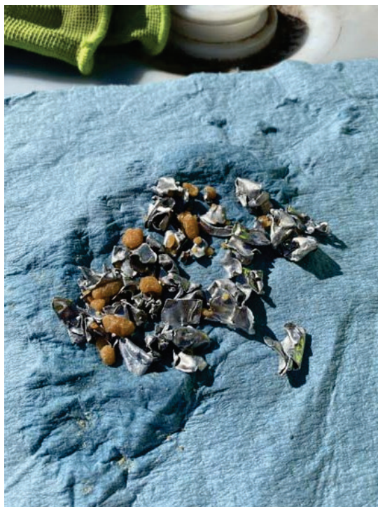
(b) Pieces of the aluminum booster cup recovered from the Cut and Capture Head
