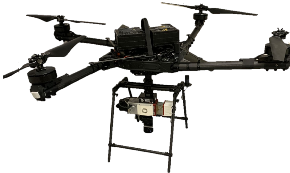
Figure 7. Alta X with LiDAR and camera payload
