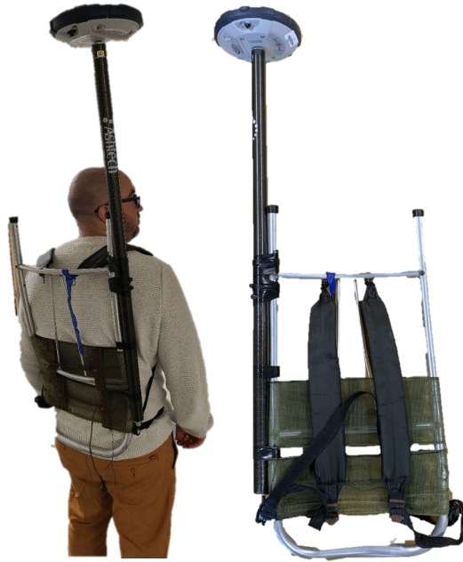
Figure 6. Survey backpack with GNSS
