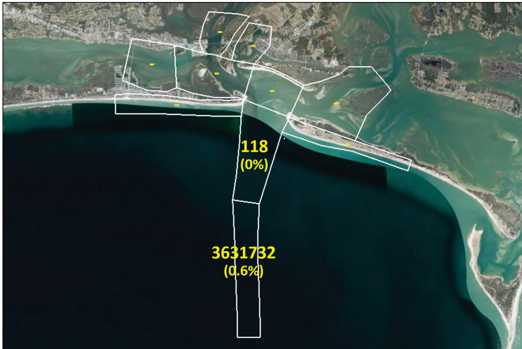
Figure 4-30. Sediment total mass (kilogram) within 10 polygon (trap) areas and percentages relative to materials placed at the ODMDS site in December 2018.
