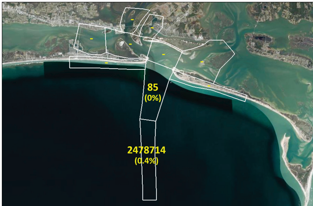
Figure 4-19. Sediment total mass (kilogram) within 10 polygon (trap) areas and percentages relative to materials placed at the ODMDS site in August 2020.
