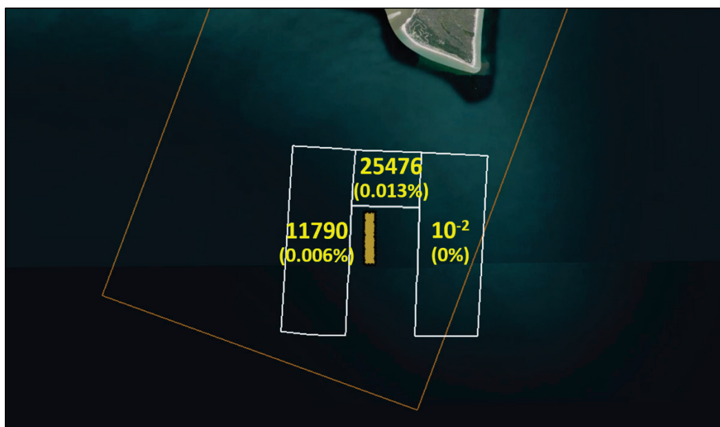
Figure 4-12. Sediment total mass (kilogram) within three polygon (trap) areas and percentages relative to materials placed at the ODMDS 1 site ( light-brown rectangle ) in June 2016.
