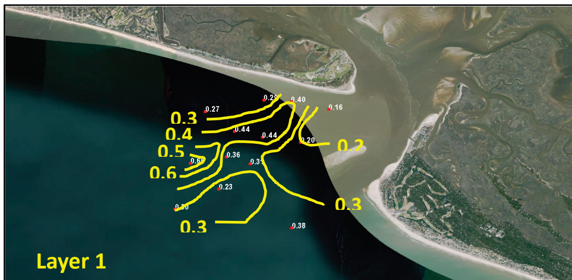
Figure 2-6. Location of sediment grab samples and contours of median grain size, D50 (millimeter).
