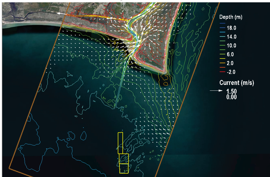
Figure 4-7. Calculated flood currents on 6 June 2016 at 00:00 (GMT). The yellow polygons indicate the dredged material placement sites.
