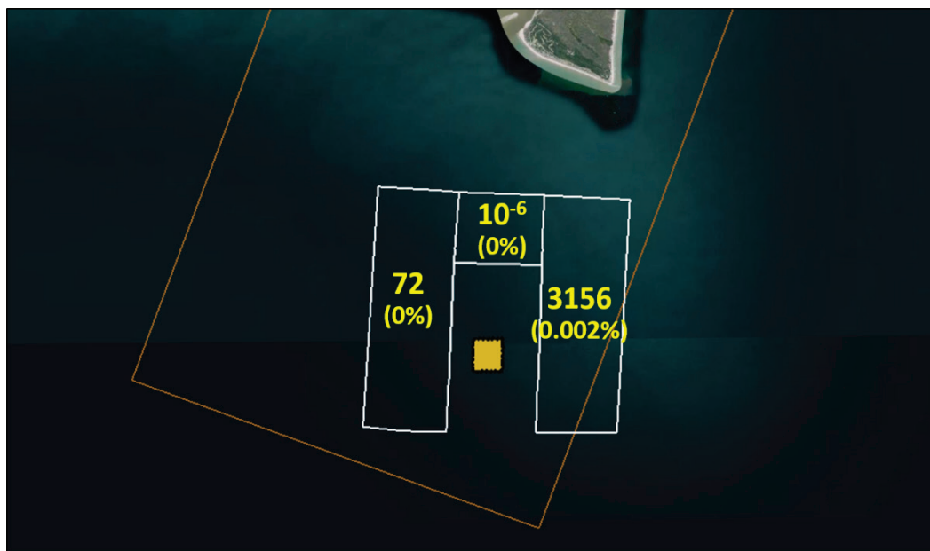
Figure 4-25. Sediment total mass (kilogram) within three polygon (trap) areas and percentages relative to materials placed at the ODMDS 2 site ( light-brown square ) in December 2017.
