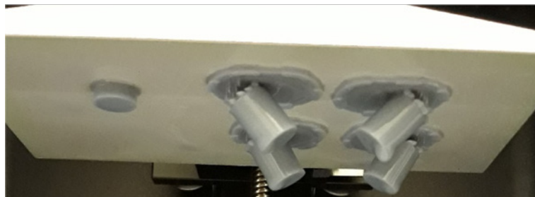
Use of supports and drainage angles.
