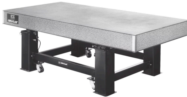
Figure 6. Kinetic Systems Inc. 5300 Series optical table. Source: [9].
