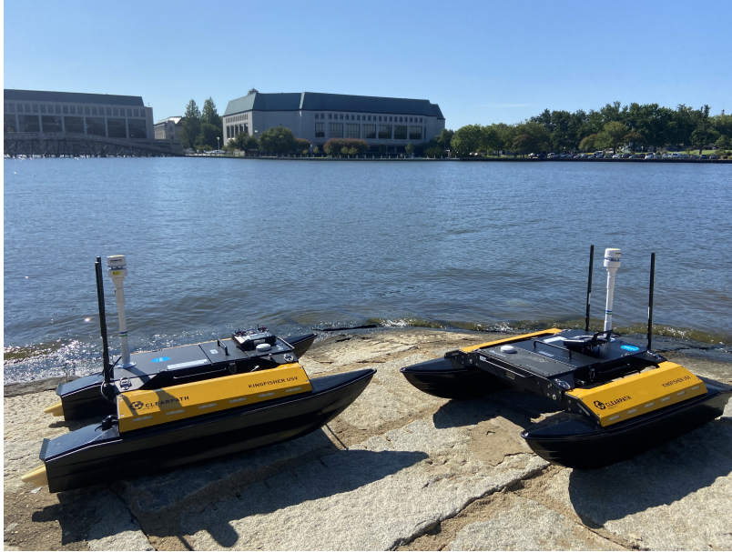
Figure 2.3. Clearpath Robotics Kingfisher M200 on shore.
