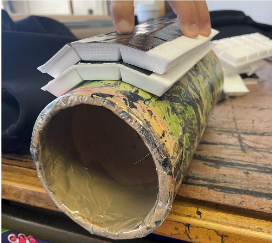
Figure 8. The white pieces in the image are the composite pieces which are double stacked over a cardboard tube showing how the composite pieces will fit over a body part. Source: [15].
