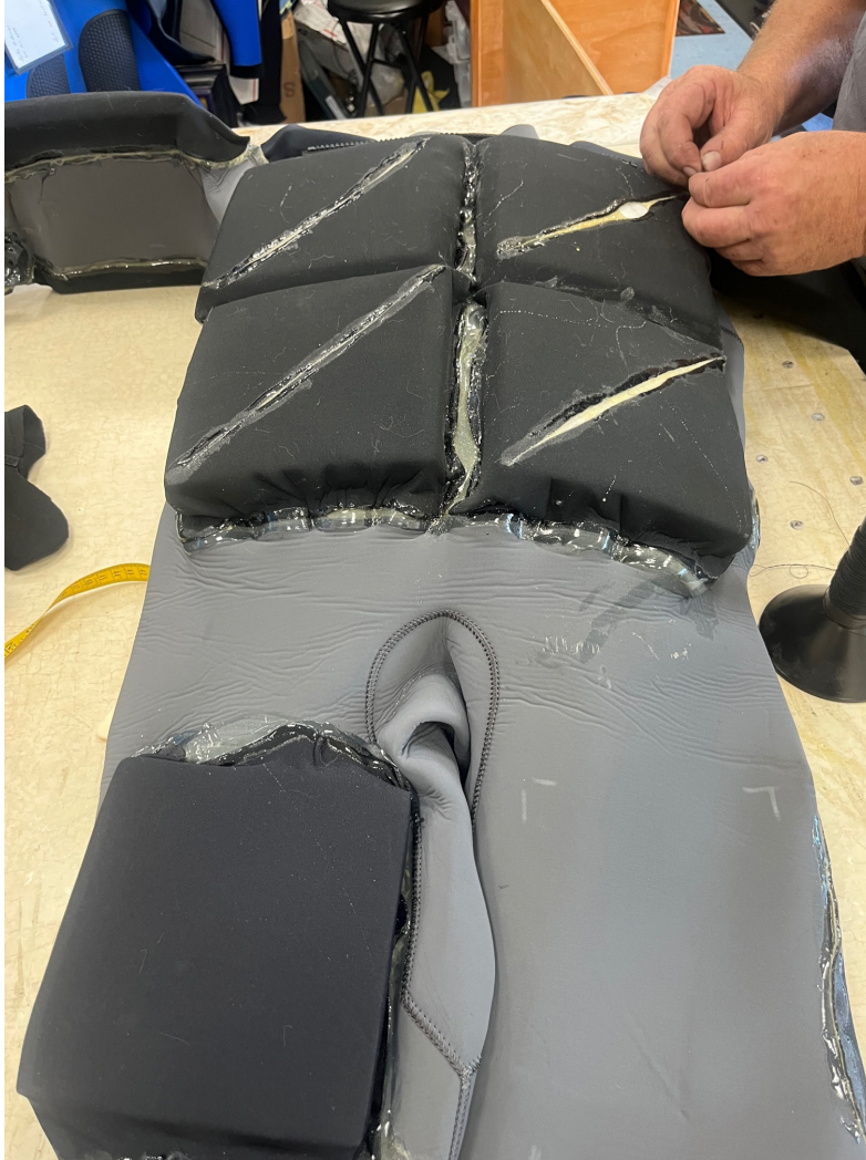
Figure 15. The neoprene wetsuit base is shown in grey. The black pieces are the pockets that are glued onto the wetsuit. The chest pieces were inserted through the diagonal cut in the pocket neoprene. The neoprene was then sewed back together using a baseball stitch and Aquaseal was then applied over the stitch to ensure a watertight seal.
