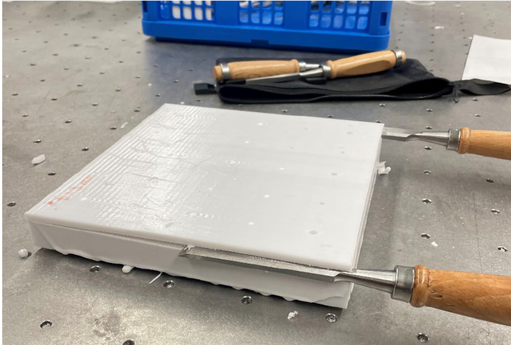
Figure 14. Chisels are used to delicately remove the top piece from the bottom mold to maintain the integrity of the composite piece. Source: [15].
