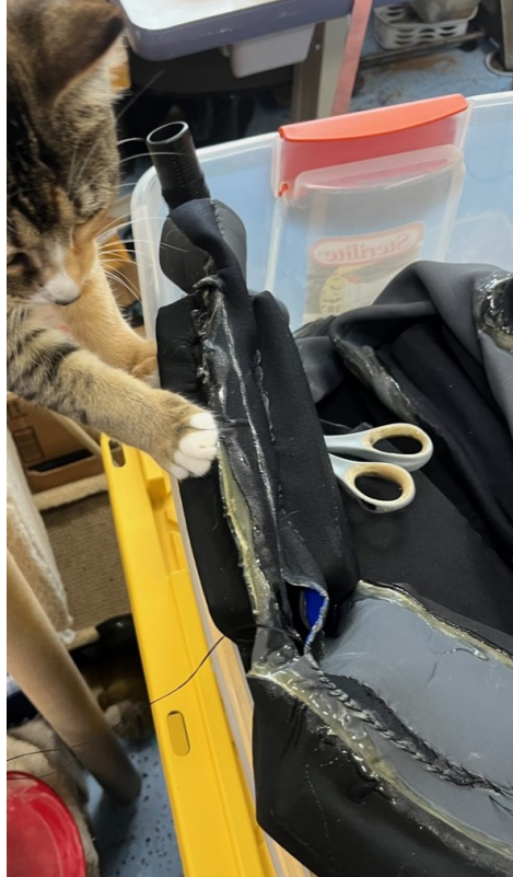
Figure 19. A depiction of how the neoprene is stitched together to patch the hole in the arm. The grey color represents the 3mm neoprene suit, while the black corresponds to the outer covering of the pockets that contain the composite pieces. This photo was taken at Otter Bay Wetsuits, with the shop cat visible in the background.
