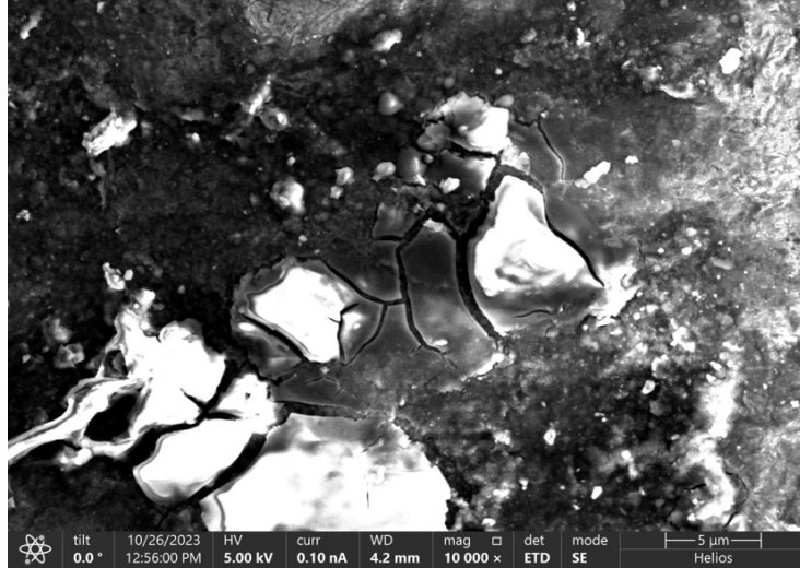
Figure 36. SEM top-down image of dual pass 2 vol% nB 4 C / 2 vol.% BNNT.
