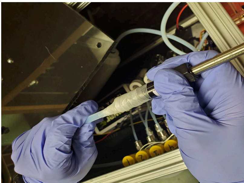
Figure 28: A) Olfactometer six-channel solenoid valve manifold. B) Solid phase microextraction (SPME) fiber olfactometer sampling procedure.
