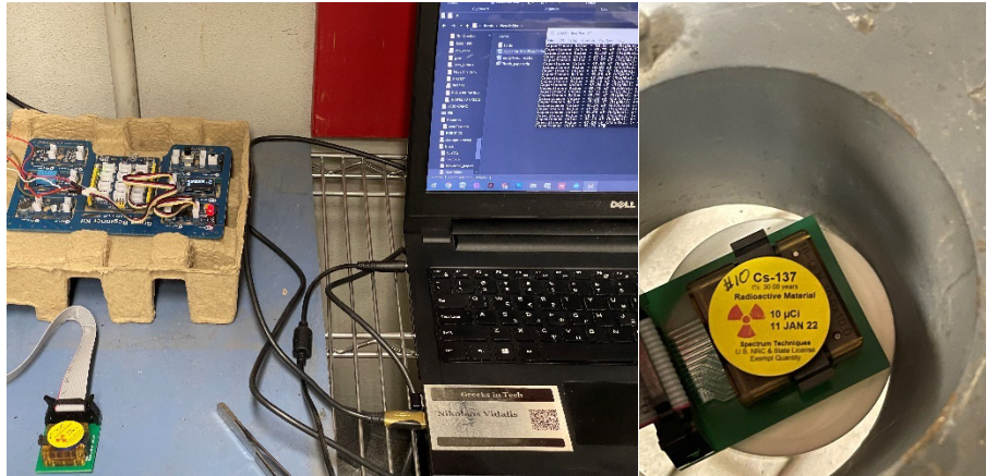
Figure 13. Measuring configuration. a) Measuring platform, b) Cs-137 disk on clamshell chip testing box
