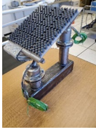
Figure 2: Heat Exchanger (HX) system
