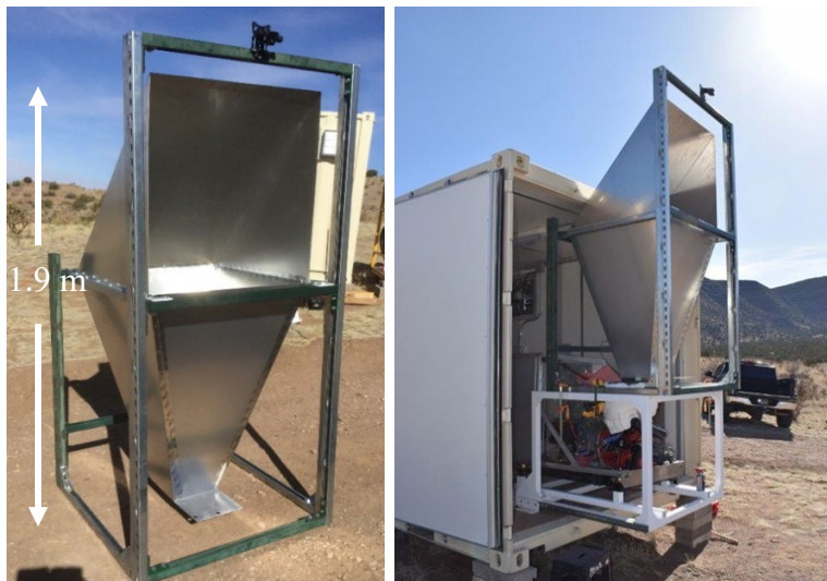
Figure 3: Beam Hopper (left) and after integration with HX & Stirling System. The Beam Hopper dimensions are 1.9 m high by .84 m wide
