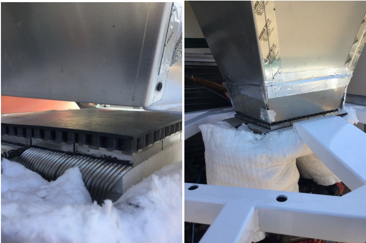
Figure 6: CLT imaging target placed on top of HX absorber cylinders. On Day 1 testing, note large gap between CLT/HX and bottom of beam hopper structure (left image). The gap was then corrected for the test on Day 2 (right image)
