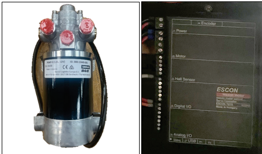
Figure 4. Simrad hydraulic pump and Maxon motor controller.
