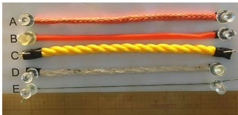
Figure 26: (a) Amsteel from Samson Rope, (b) 550 parachute cord, (c) Polypropylene line, (d) Fibrous cotton rope, (e) braided fishing line (200-lb test). A ruler runs along the bottom of the image
