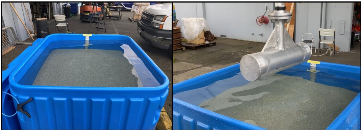
Figure 1. Laboratory Testing Tank, fluidization test target shown in right pane
