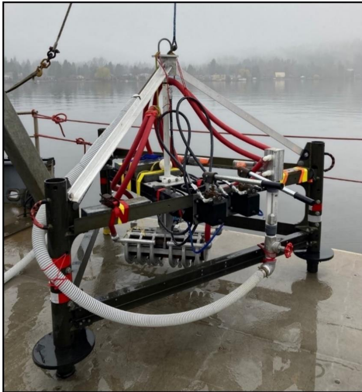
Figure 5. Bottom lander frame with manipulator, water hoses and hydraulic controls
