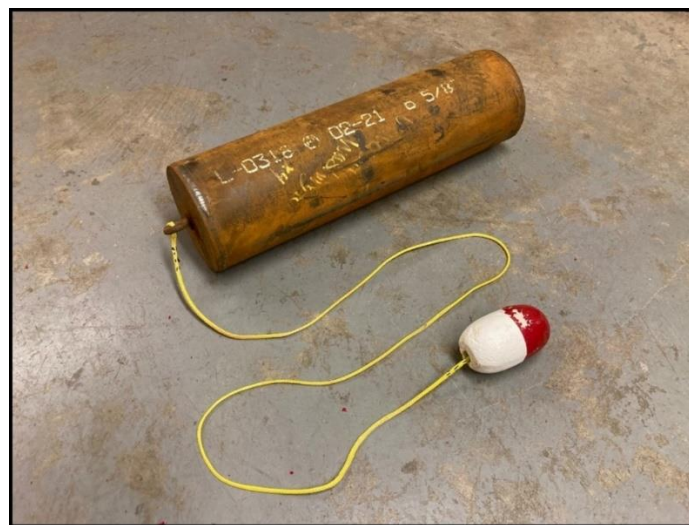
Figure 8. Field testing burial target with marking/lifting line and float
