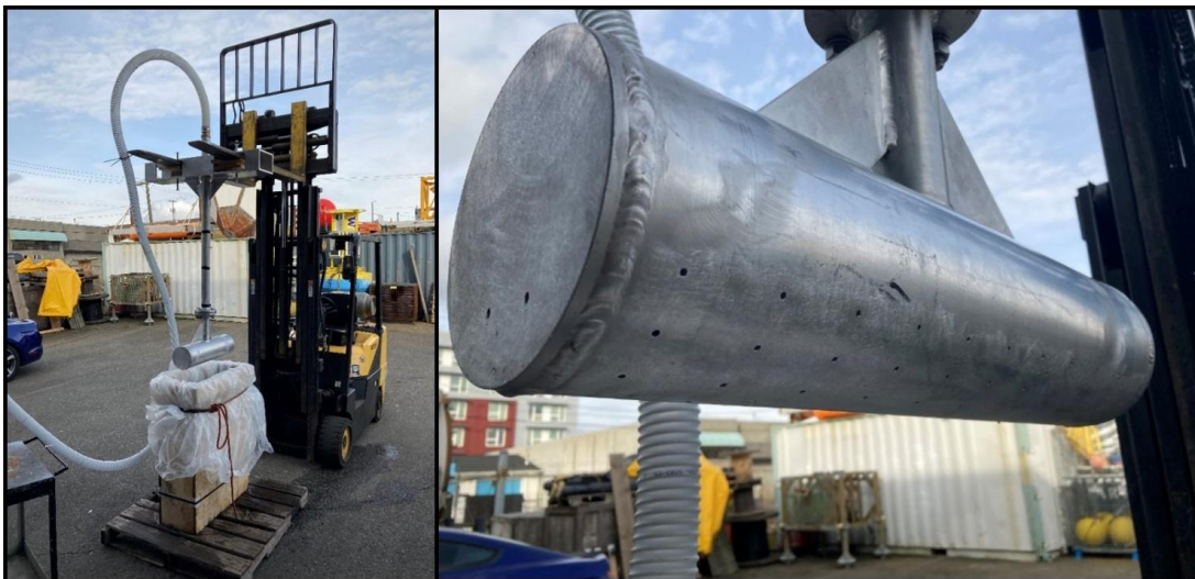
Figure 2. Laboratory fluidization and burial target. Fluidization jet holes shown in the right pane
