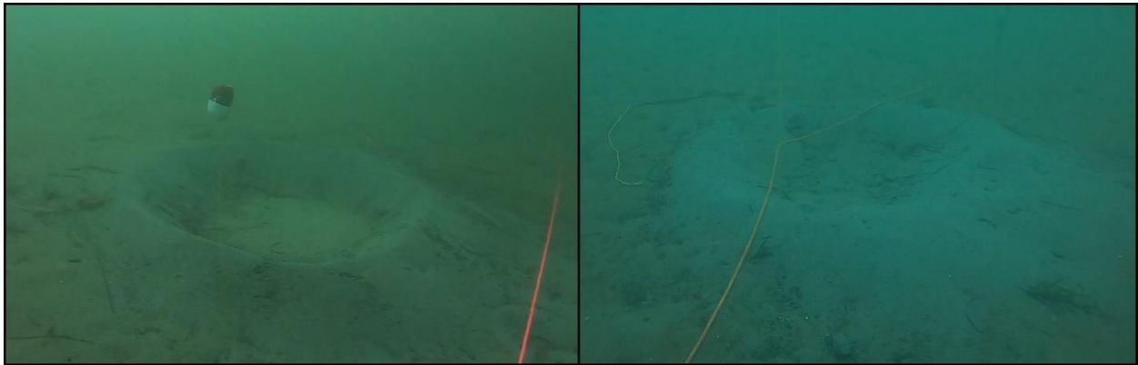
Figure E 5. Target burial crater immediately after burial (left) and again one week later (right)
