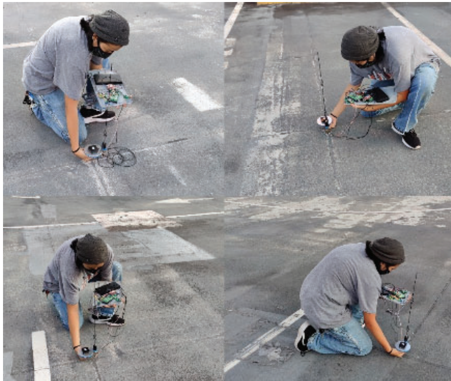
Figure B.8. Placing the RTK Module Antenna at Each Corner.
