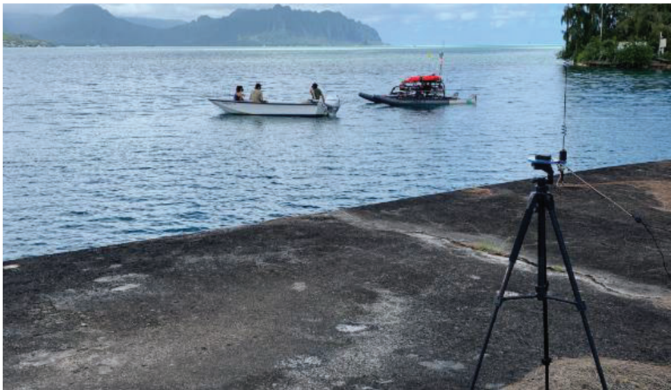
Figure 2.5. RTK GNSS Ground Station (Foreground) in View of WAM-V with Three RTK GNSS Sensors Aboard.
