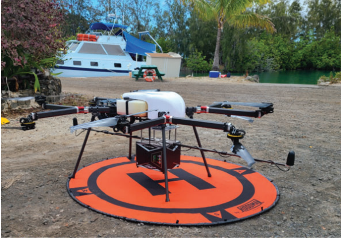
Figure 7.7. ASTRALiTe Edge Mounted Beneath the Skyfront Perimeter 8 UAV.
