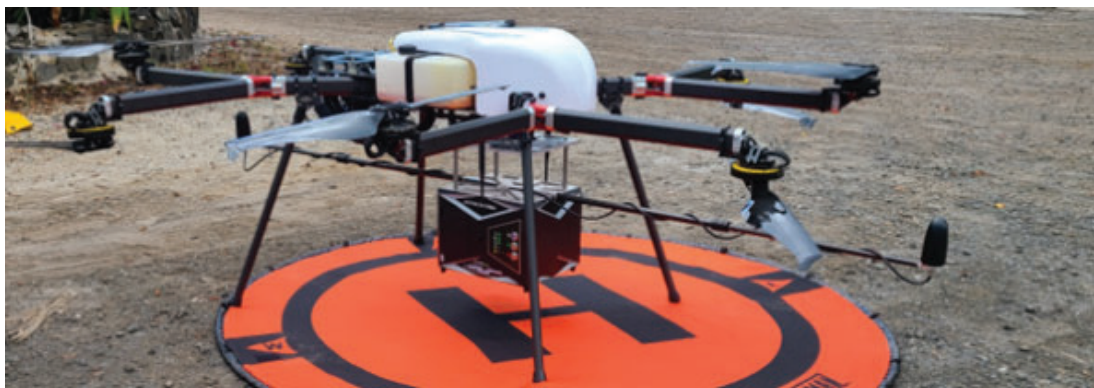
Figure 2.3. ASTRALiTe Edge Mounted Beneath the Skyfront Perimeter 8 UAS.
