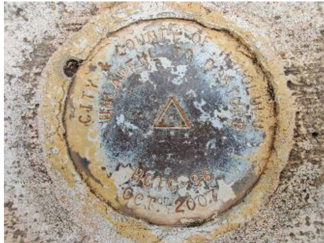
Figure B.3. HCTC 96 NGS Geodetic Marker.
