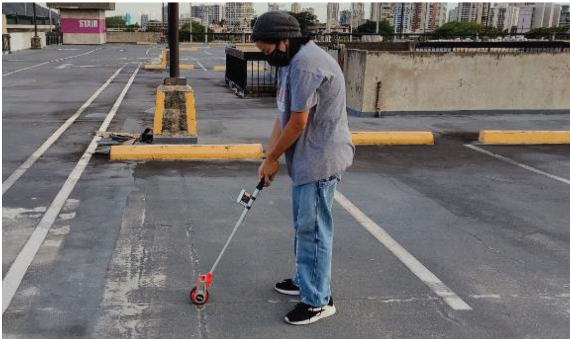
Figure B.9. Wheeled Measuring Tool Used to Measure the Distance Between the Four Corners.
