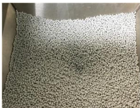
rPET pellet fully crystallized
