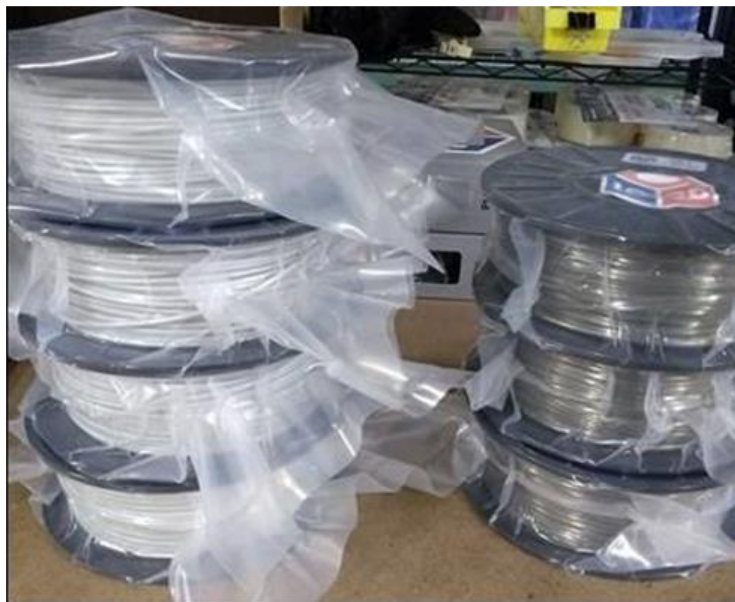
Figure 16. rPET filament spools with (opaque) and without (translucent) additive
