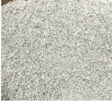
Figure 1 – Photo of clean, 4-mm rPET white flake from PET water bottles used for AM filament production trials
