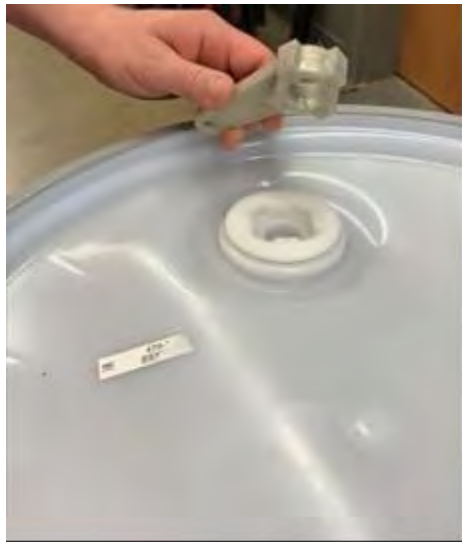
Figure 5 – Photos of the smaller 55-gallon drum wrench design printed with 2.85 mm rPET filament being used to open and close the drum.
