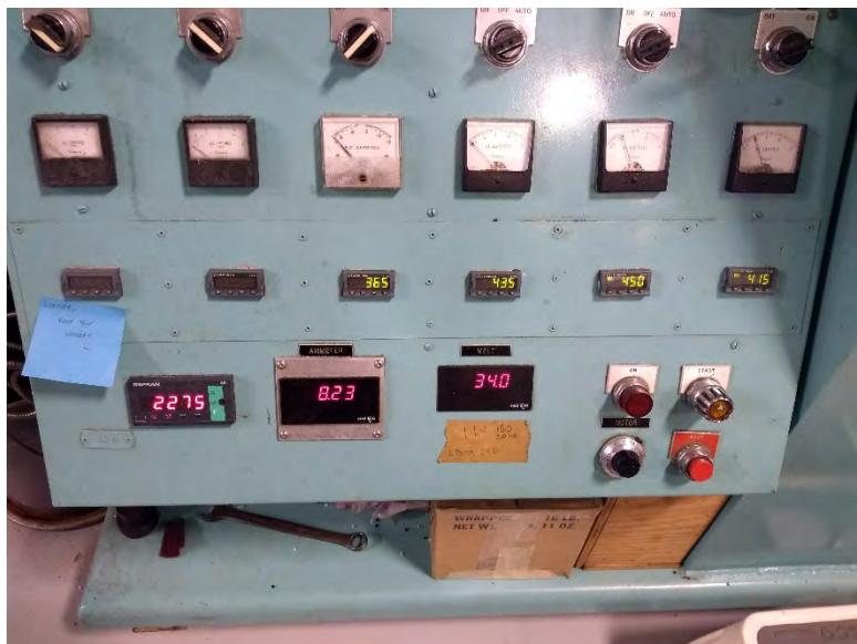
Figure 2: Extruder settings for rPET only
