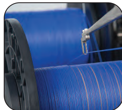
A Conair automatic cut-and-transfer coiler smoothly wraps filament onto production-size reels, ready for transfer to smaller spools in a separate operation.
