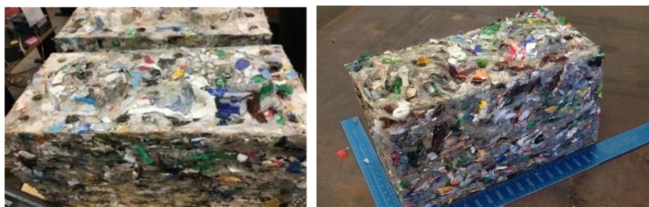
Figure 25. Photograph of typical ByBlock made with mixed plastics waste
