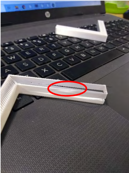
Figure A: Calibration 'L' bracket printed w/ no infill and single wall
