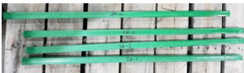
Figure 21. rPET plastic lumber (1" x 1") test specimens with green flake
