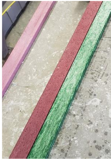
Figure 24. 2x4 rPET lumber produced with commercial flow molding equipment
