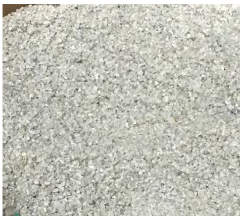
Figure 3 – Photo of rPET-White Flake Sample
