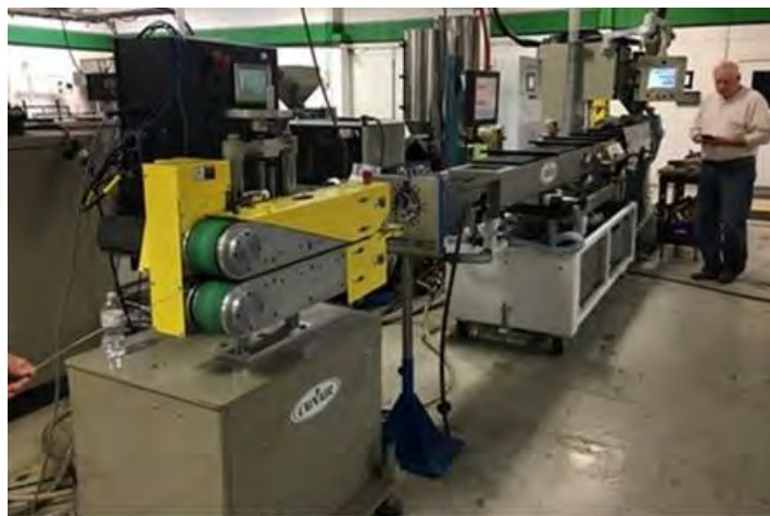
Figure 3 – Photograph of rPET 3D printer filament extrusion trials at Conair
