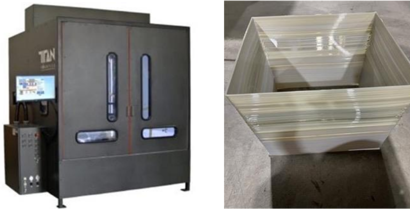
Figure 36. Photo of Titan printer and hollow box specimen printed with rPET pellets
