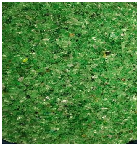
Figure 4 – Photo of rPET-Green Flake Sample
