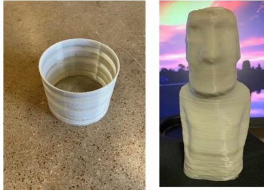
Figure 38. Calibration cylinder and ‘logo’ printed on Gigabot-X with rPET flake
