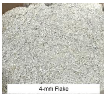
Figure ES-3 – Sample of clean 4-mm rPET flake delivered from ‘sorting and washing line’
