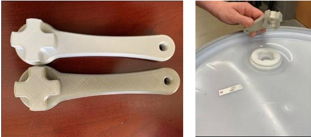
Figure 34. Drum wrench printed with both rPET filament with and without additive
