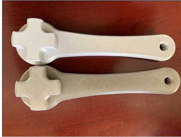
Figure 4 – Photos of 55-gallon drum wrench printed with both 2.85 mm rPET filament without additive (translucent at the bottom) and with 10% Kraton (opaque at the top)
