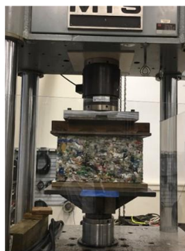
Figure 26. ByBlock samples under compression testing
