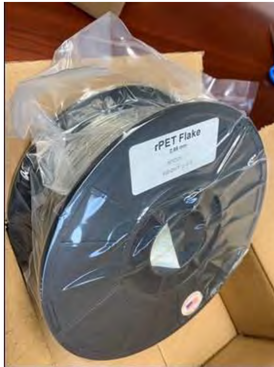
Figure 2 – Photo of 2.85 mm diameter rPET filament spool made from clean flake shown in Figure 1
