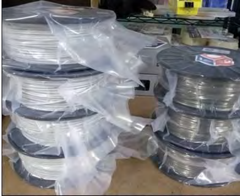
Figure 4 – Photo of IC3D trials to make 2.85 mm rPET 3D filament on commercial production equipment with additive (10% Kraton; opaque) and without additive (translucent)
