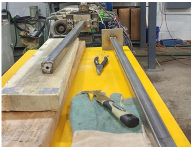
Figure 17. Molds for plastic lumber test specimens (1" x 1" x 36")
