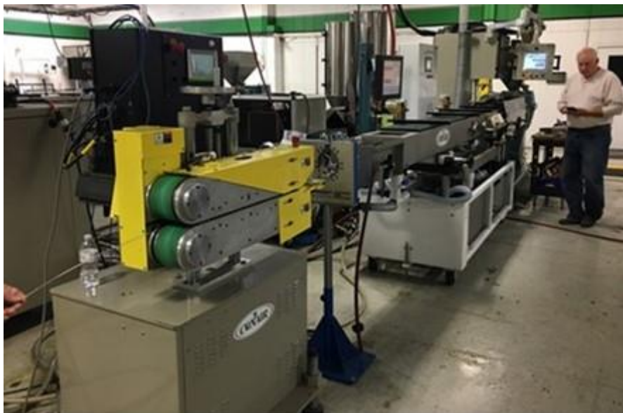
Figure 14. Photograph of rPET 3D printer filament extrusion trials at Conair
