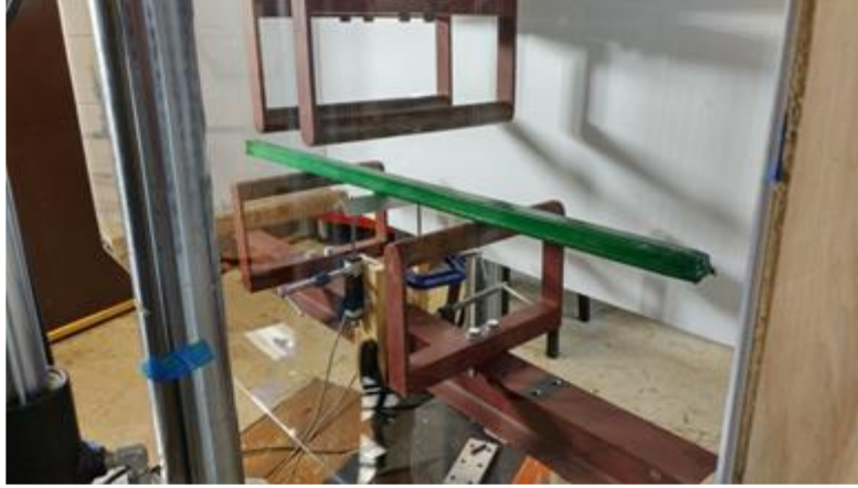
Figure 19. Four-point bend fixture for testing plastic lumber
