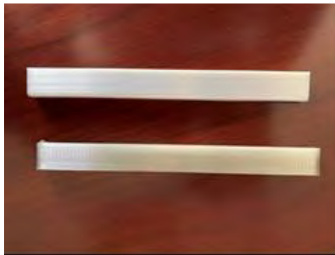
Figure 3 – Photos of ASTM D 790 (Flexural) specimens printed with both 2.85 mm rPET filament without additive (translucent at the bottom) and with 10% Kraton (opaque at the top)
