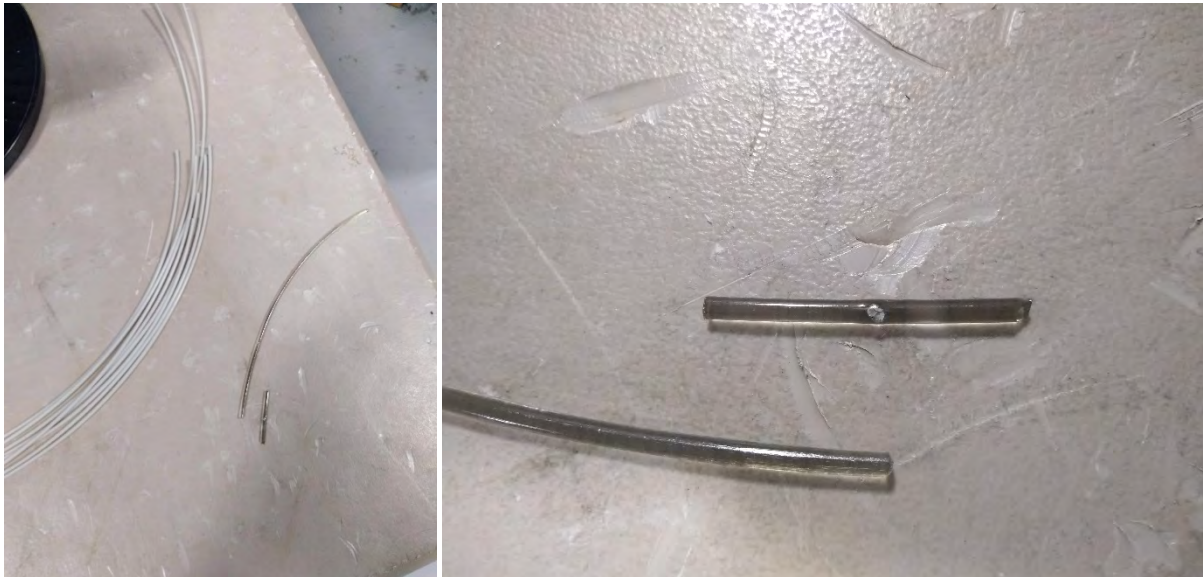
Figure 3: Left shows overdiameters removed in post extrusion quality check – rPET alone had far less problems. Right shows closeup of extrusion contaminant from rPET regrind process –appears to be aluminum
