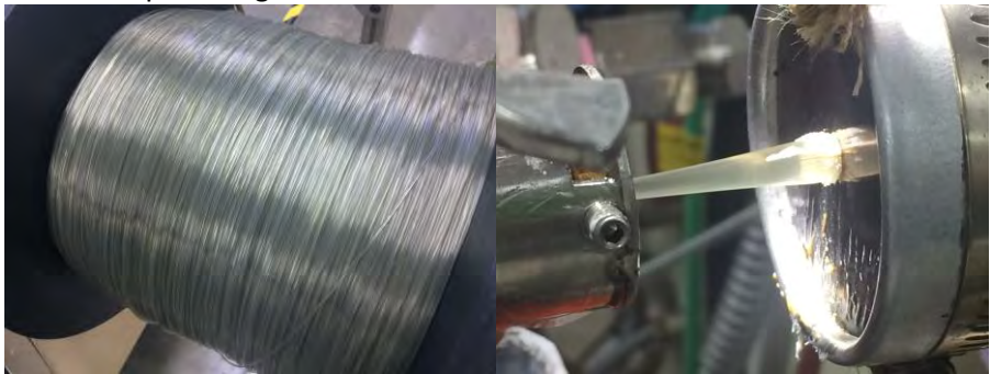
4:17 Die build up starting to occur
