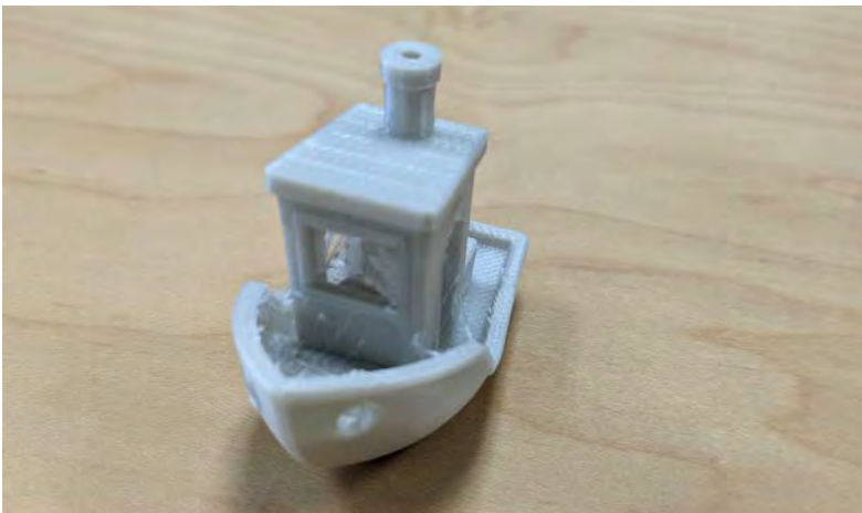
Figure C: Benchy front view showing close-up of stringing. Filament has excellent bridging characteristics and captures detail well with given settings
