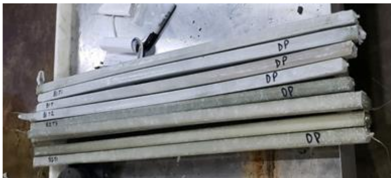
Figure 18. rPET plastic lumber (1" x 1") test specimens with white flake
