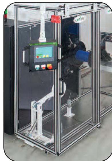
A Conair automatic cut-and-transfer coiler smoothly wraps filament onto production-size reels, ready for transfer to smaller spools in a separate operation.
