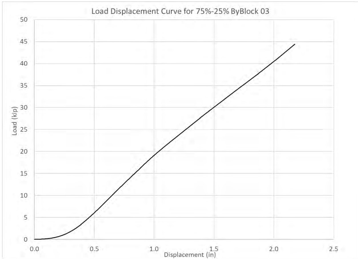
Figure 5: Load Displacement Curve for 75PET25HDPE03
