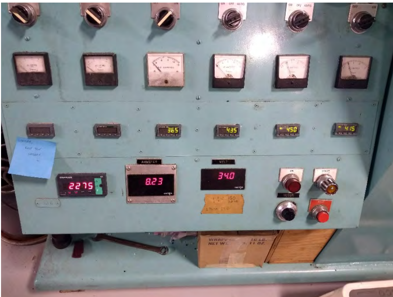
Figure 2: Extruder settings for rPET only
