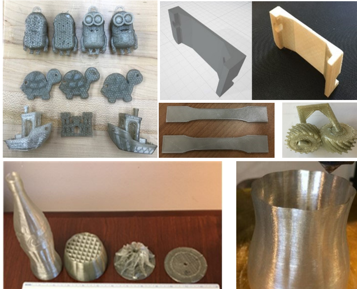
3D-printed samples, ASTM specimen and 90-degree transmission gear from rPET filament
