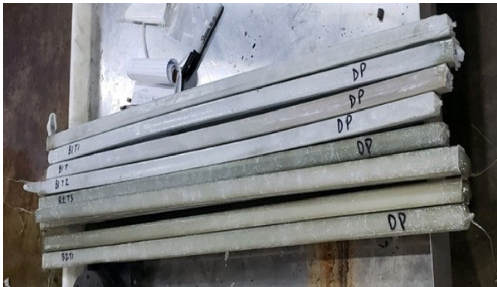
1-inch x 1-inch x 36-inch specimens
