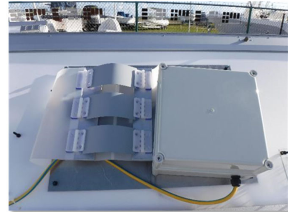
Deployment of apparatus for flexing coated aluminum 2024-0 alloy panels during outdoor exposure on 45° inclined exposure rack on Fleming Key, FL.
