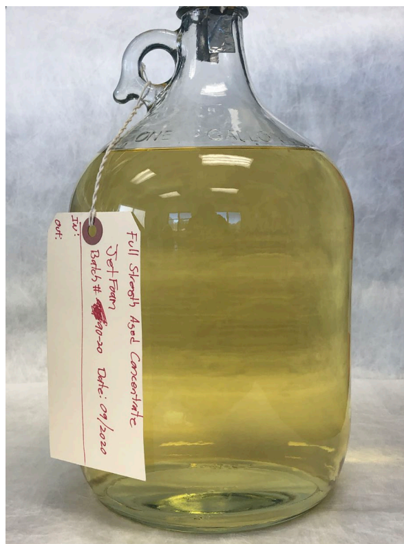
Figure-2: Angus Fire Jetfoam 3% Aged Concentrate Sample
