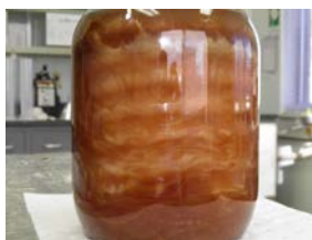
Figure-5: Solberg RF3 Aged Concentrate (NRL-CBD Testing, December 2019)
