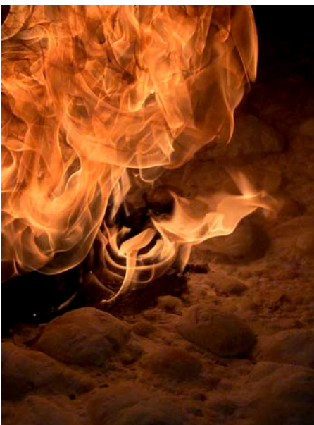
Figure-4: Solberg RF3 PKP Jet Fuel (JP-8) Compatibility Test (Formation of an Unusual Black Substance in the Foam Blanket outside the Burnback Test Pan)
