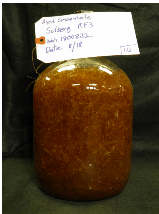
Figure-1: Solberg RF3 Aged Concentrate Sample
