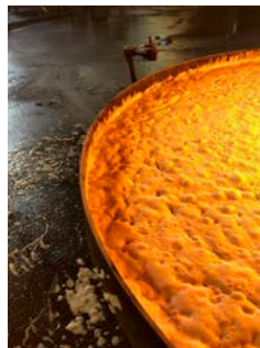
Figure-3: Solberg RF3 Ethanol-Free Gasoline PKP Compatibility Test (Foam Degradation along Fire Test Pan Perimeter)
