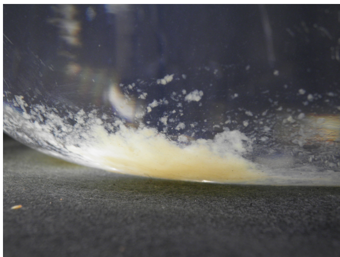
Figure-5: Fomtec ENVIRO USP 3% Aged Pre-Mixed Solution Noting Sediment
