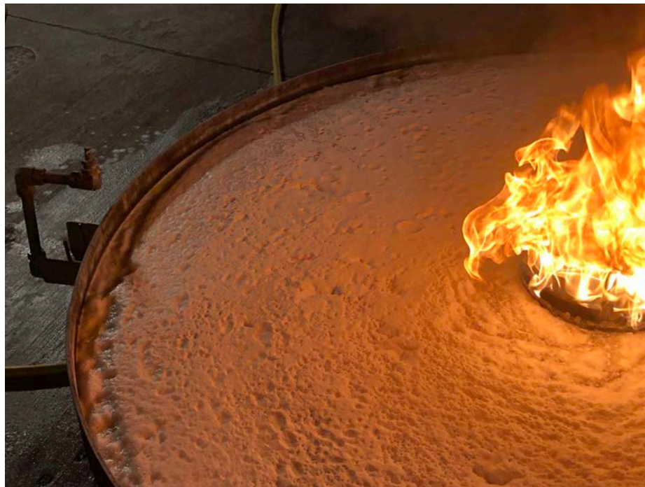
Figure-1: BioEx ECOPOL A 3% PKP Compatibility Test (Foam Degradation along Fire Test Pan Perimeter)
