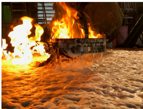
Figure-1: Fomtec ENVIRO USP 3% Quintuple Strength Burnback Test
