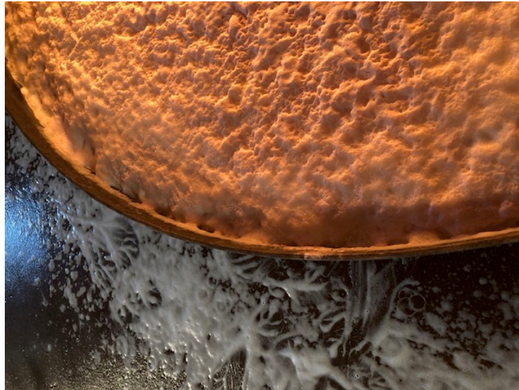
Figure-3: AVIO F3 Green KHC 3% PKP Compatibility 28ft 2 Gasoline Fire Test
