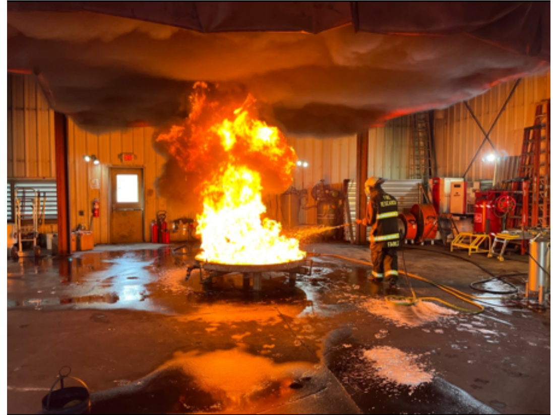
Ignited fuel in 28 ft 2 pan, Application of foam-additive mixture
