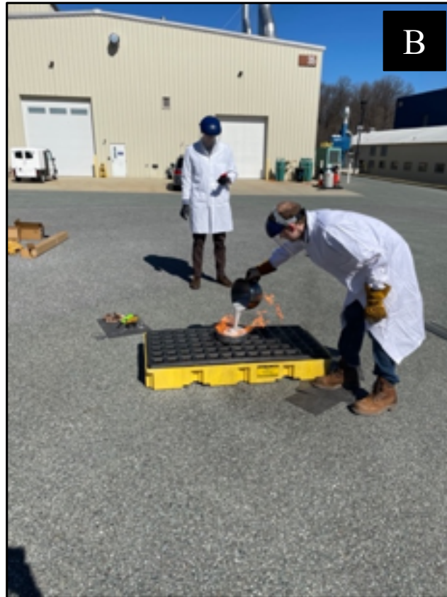
Pouring foam mixture over fire, measuring time to extinguish
