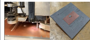
Milling machine etching out copper-plated antenna on substrate
