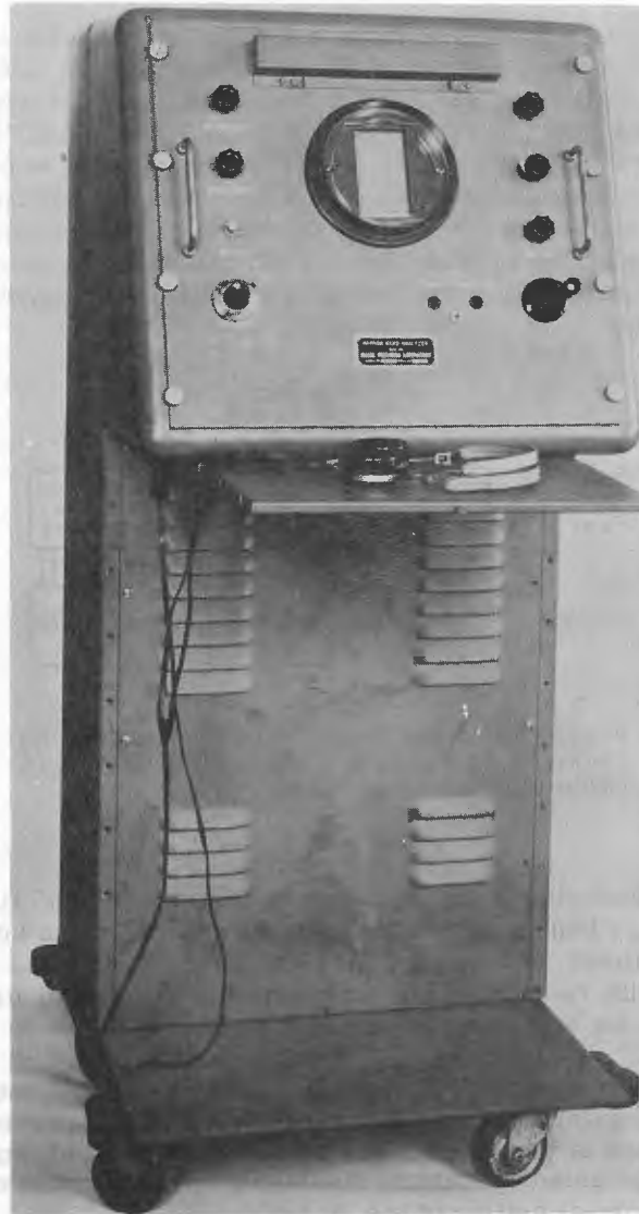
Fig. 6 - Frequency-scanning receiver, Model III (Unclassified)
