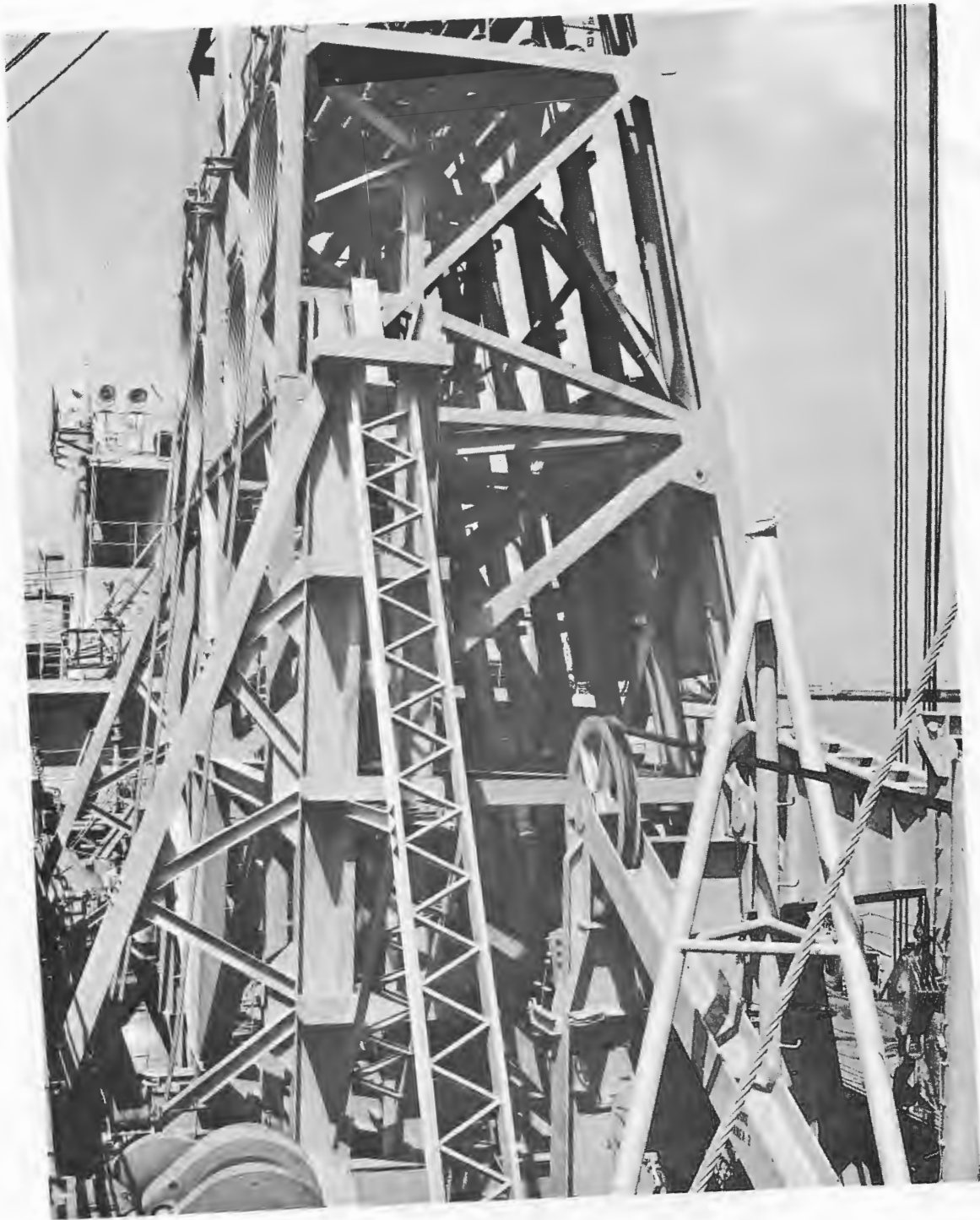
Figure 73 - Array structure in elevated position viewed from aft
