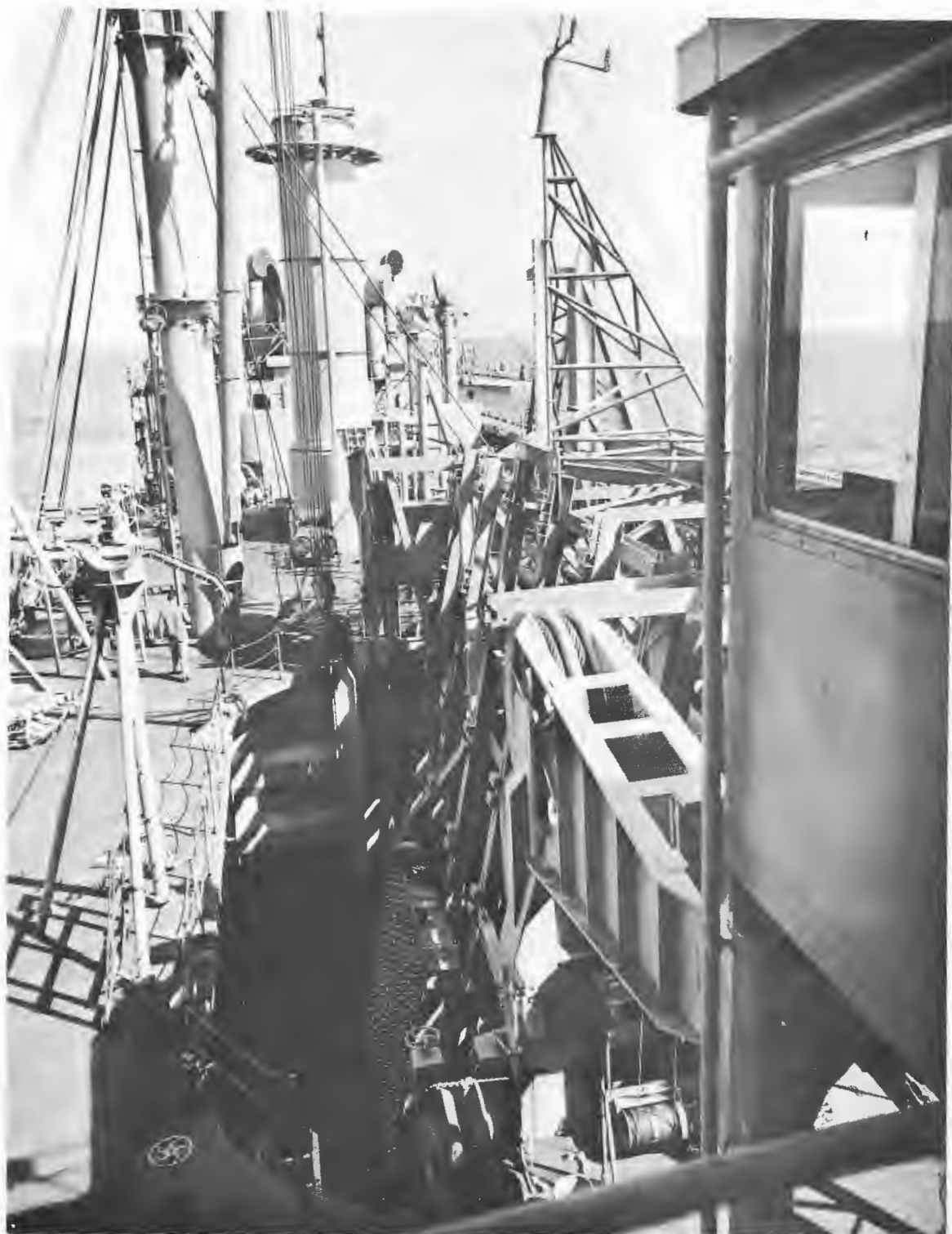
Figure 78 - Transducer array structure in stowed position
