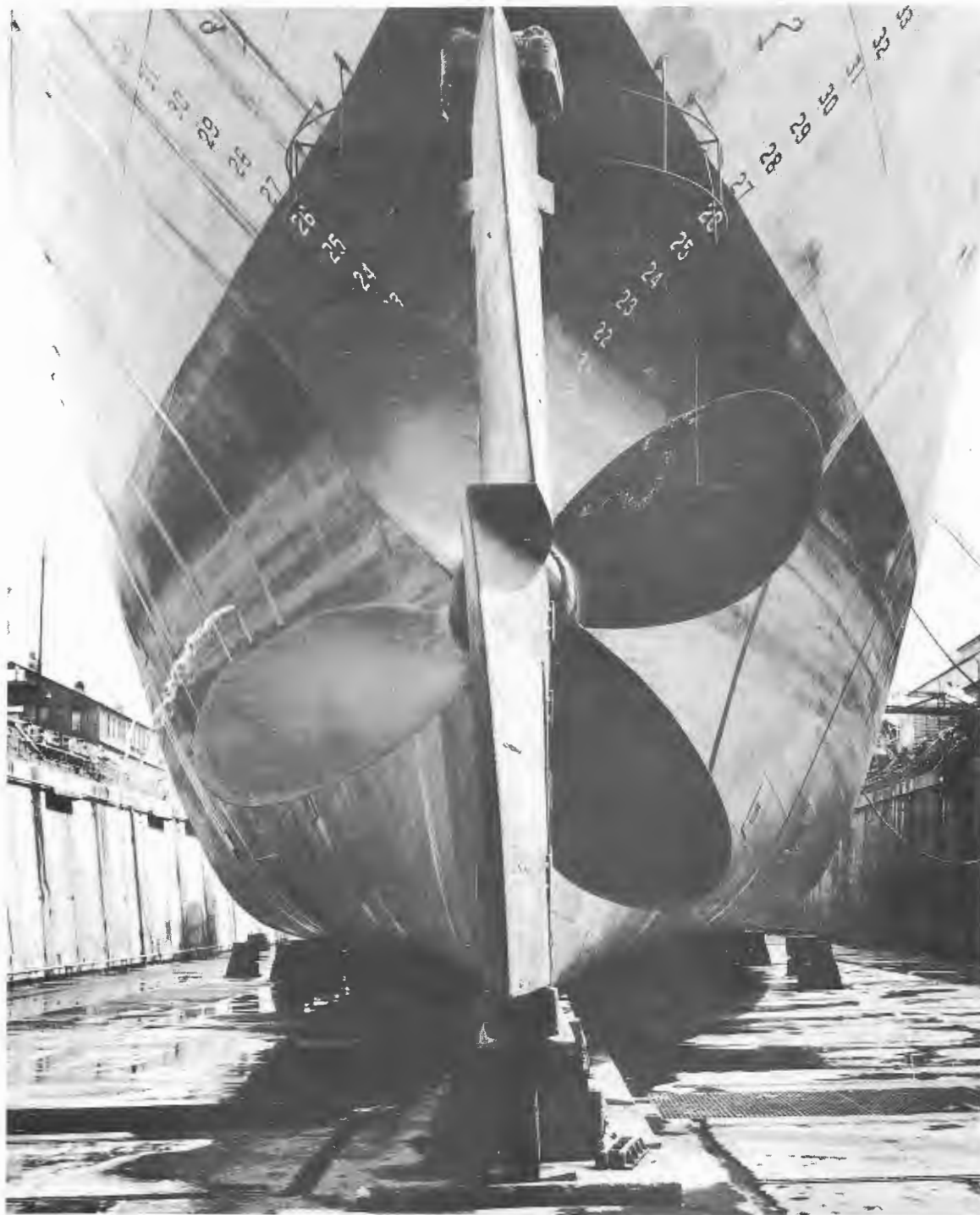
Figure 8 - Blocking arrangement viewed from stern
