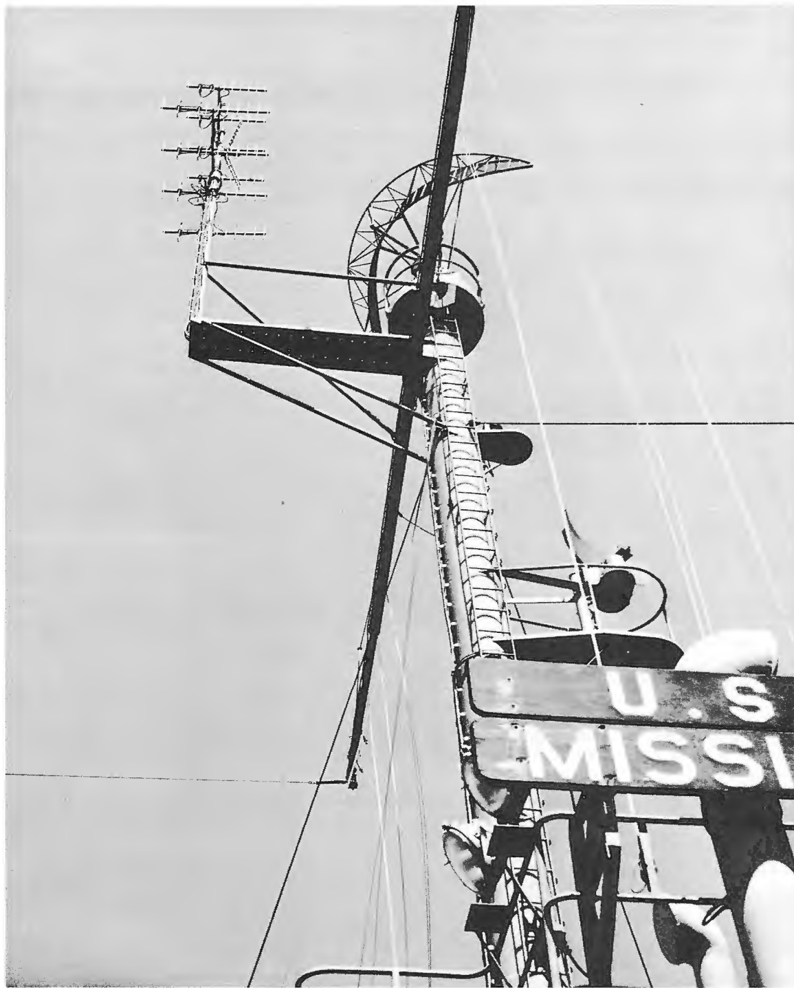
Figure 10 - Main mast with ship's radar antenna and special yagi antenna for project equipment as seen from starboard side, 02 level
