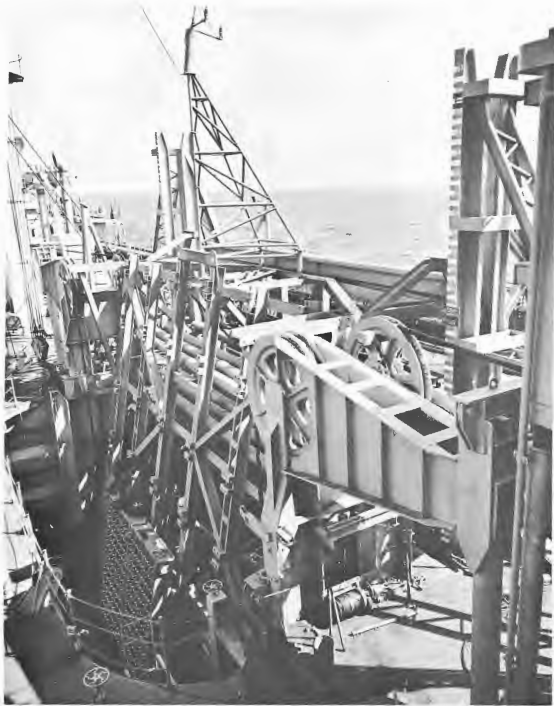
Figure 79 - Transducer array structure in stowed position
