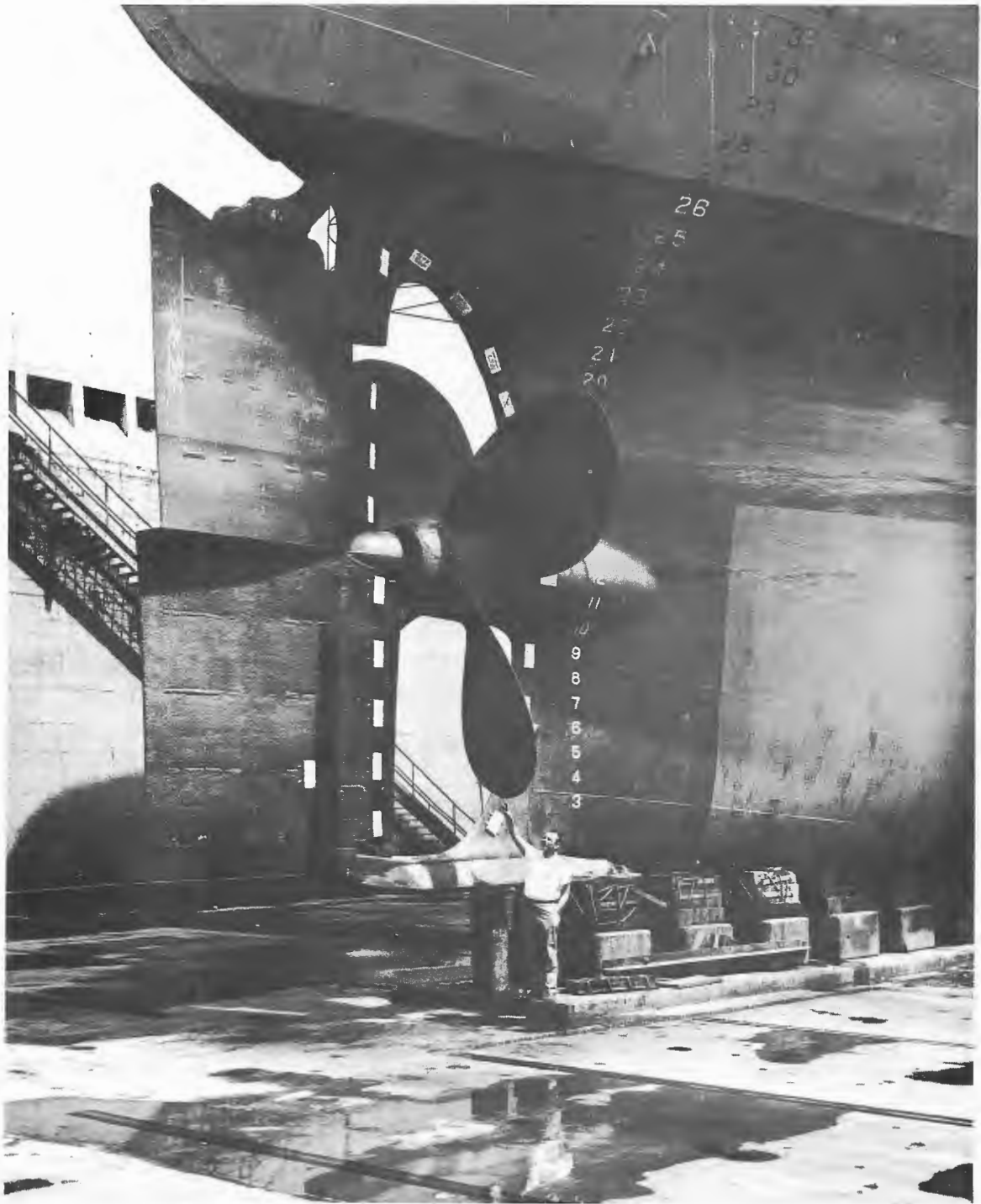
Figure 9 - Anodic protection of rudder and hull at stern
