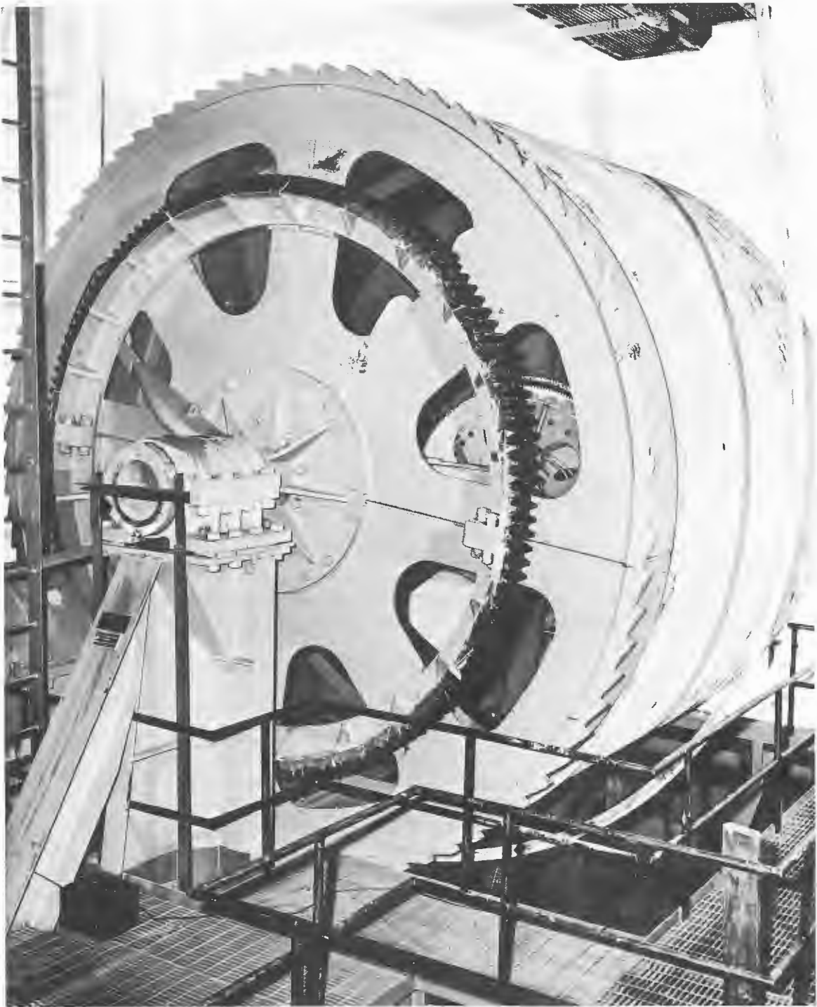
Figure 53 - Electric cable winch for instrumentation cable
