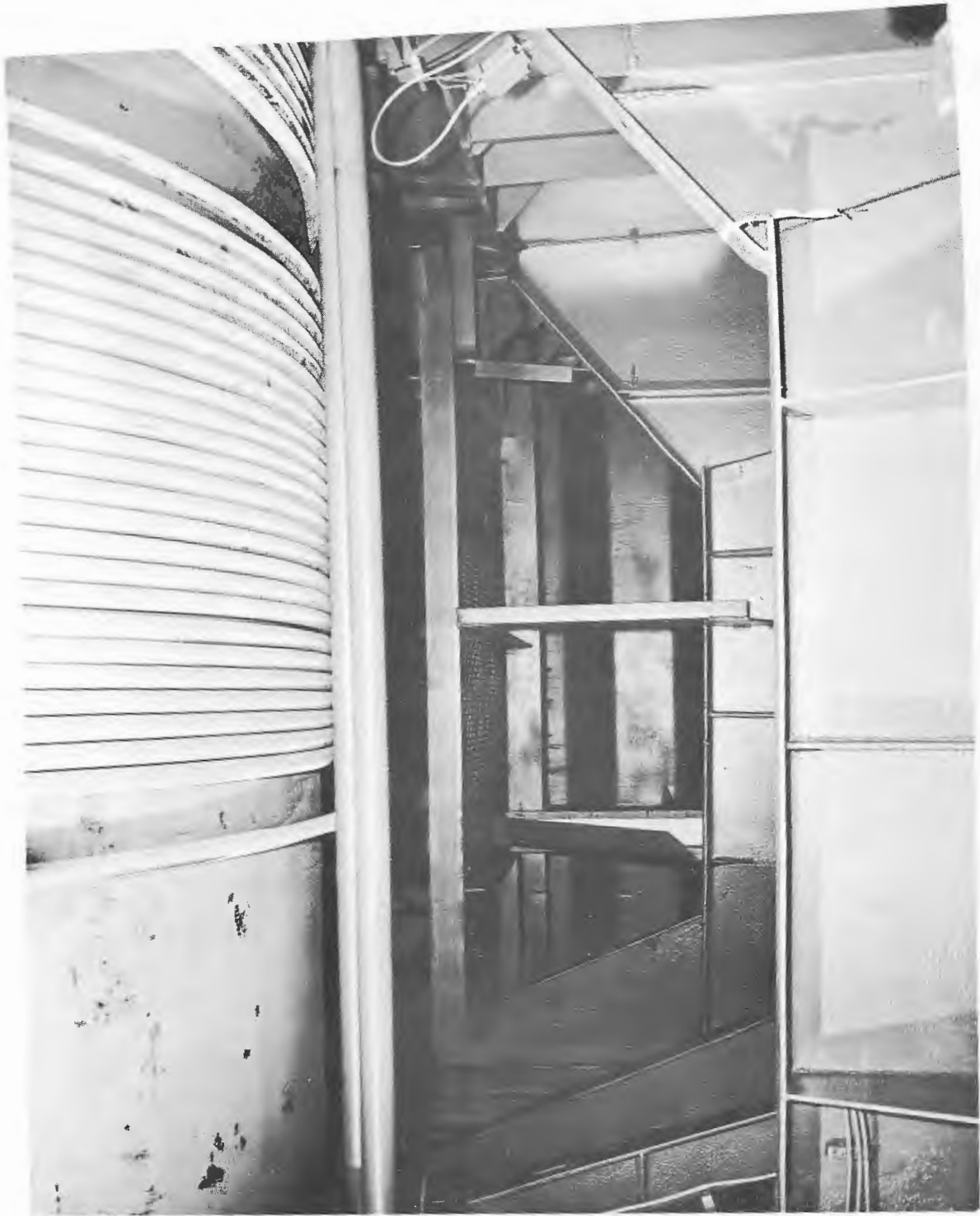
Figure 58 - Electric cable winch, drum and slack cable indicator bar
