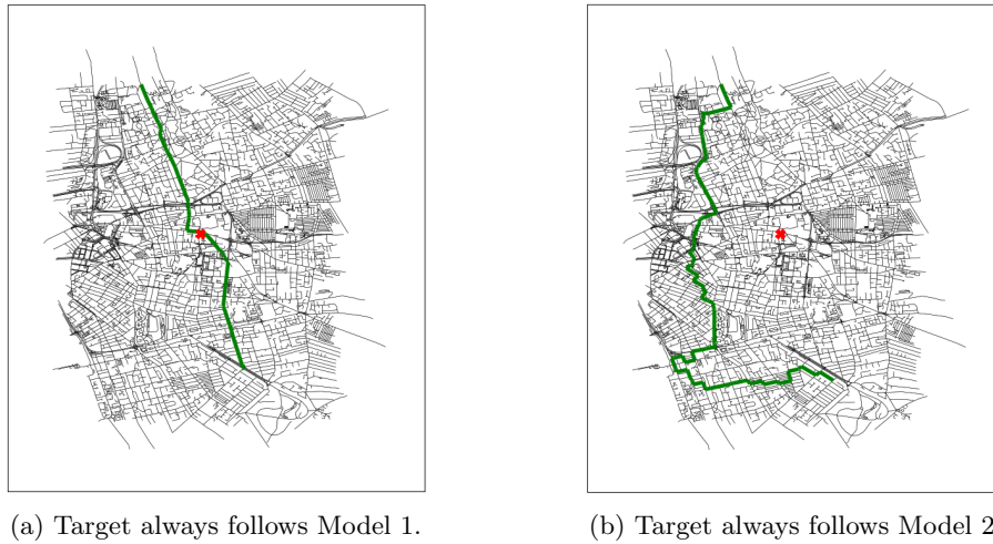
Figure 3.4: The true path (green) of the target following two models. The position of the sensor is marked by the red cross. Note that the source node is located at the Northern end of the map and the true destination node is located towards the Southern end of the map.
