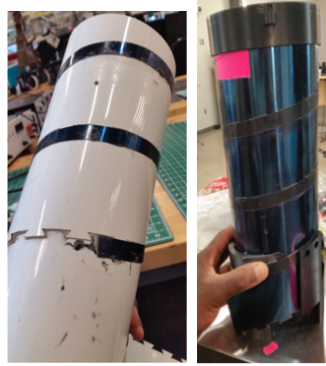
Figure 2.5: Compression test results showing backing failures with plastic and metal bands and backing.
