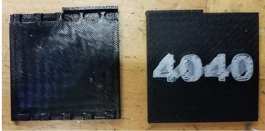
Figure 2.7: An example of one of the ABS cold forming dies. The plastic dies would begin to wear after two or three uses on 0.005" thick bronze.
