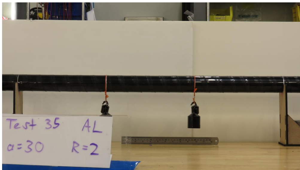
Figure 2.15: A spiral zipper column subjected to four-point bending in the test rig.
