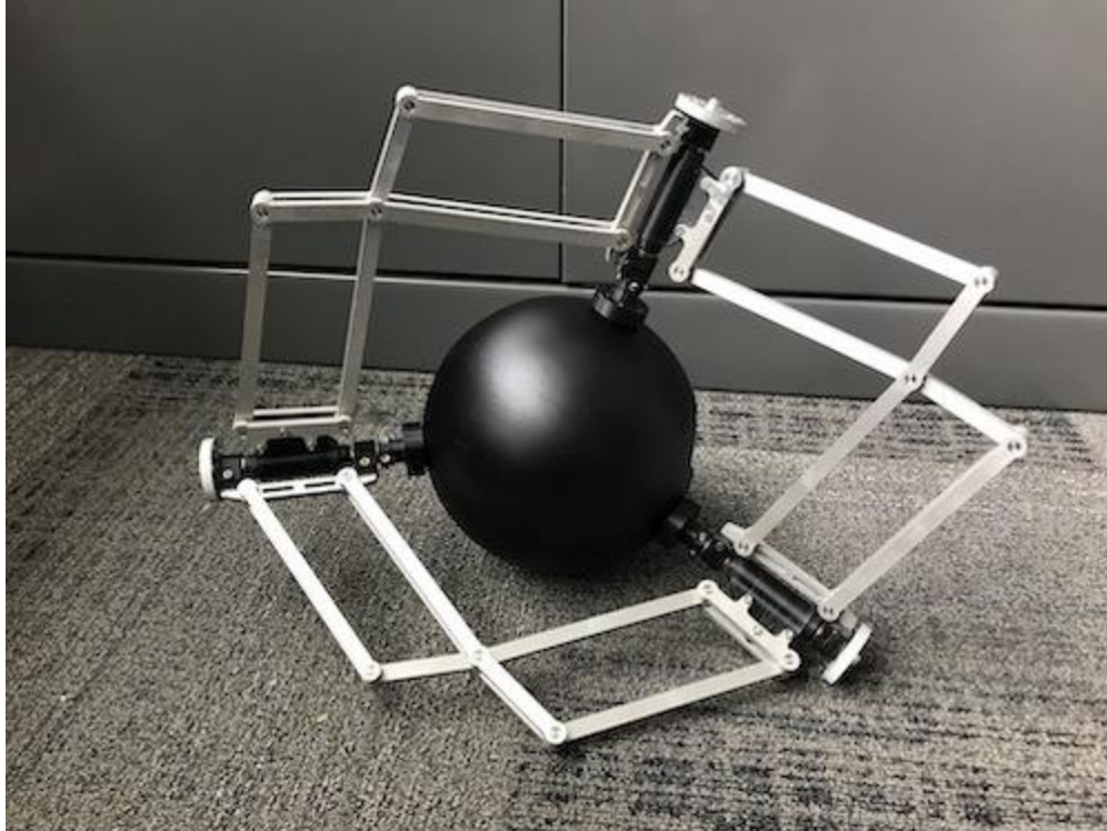
Figure 2.40: A chain of three passive six-bar linkage joints.
