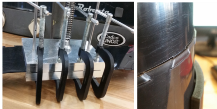
Figure 2.6: Thermoforming the band using heated dies (left) and the resultant structure (right).
