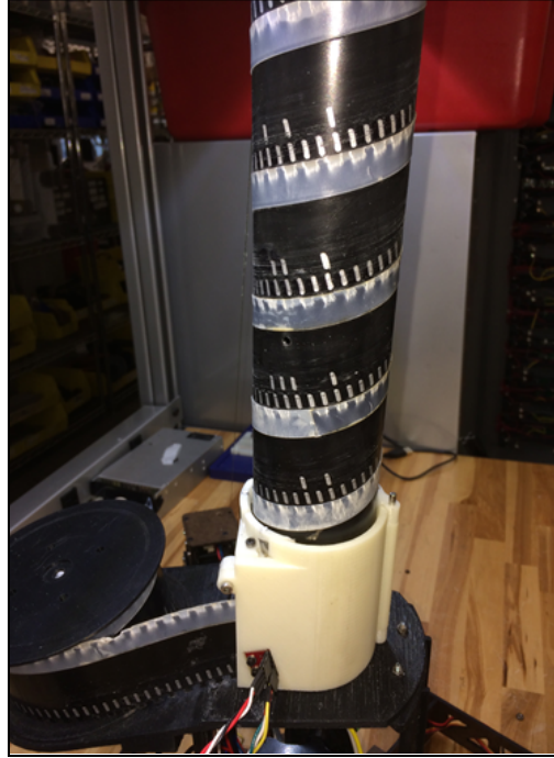
Figure 2.14: The spiral zipper with light sensor and encoder markings. Originally marked on the zipper with a permanent marker, we now use printed stickers.
