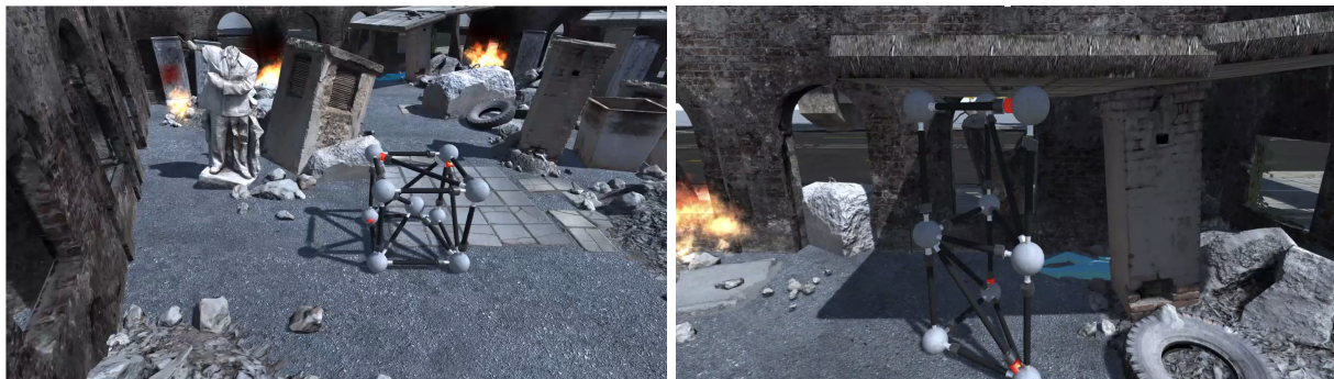
Figure 1.1: A concept simulation (from collaborators at SNU) that shows a VTT system in a disaster scenario entering a hotzone via a tumbling gait (a) and shoring a partially collapsed structure (b).
