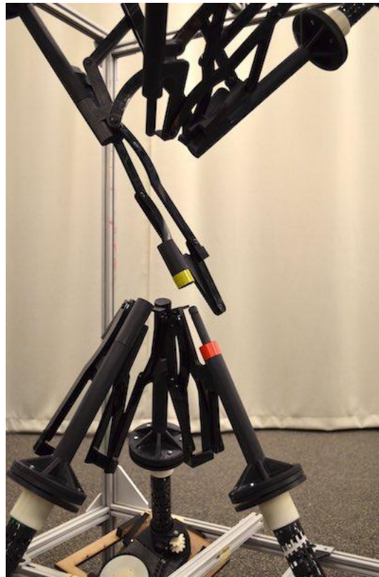
Figure 2.35: A demonstration of the “chain of joints” concept to merge and split two nodes.
