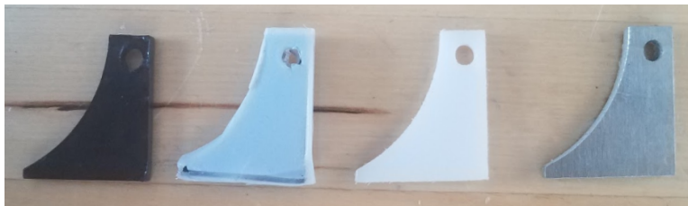
Figure 2.28: Examples of wear inserts (left to right: ABS, ABS + PTFE, HDPE, aluminum).
