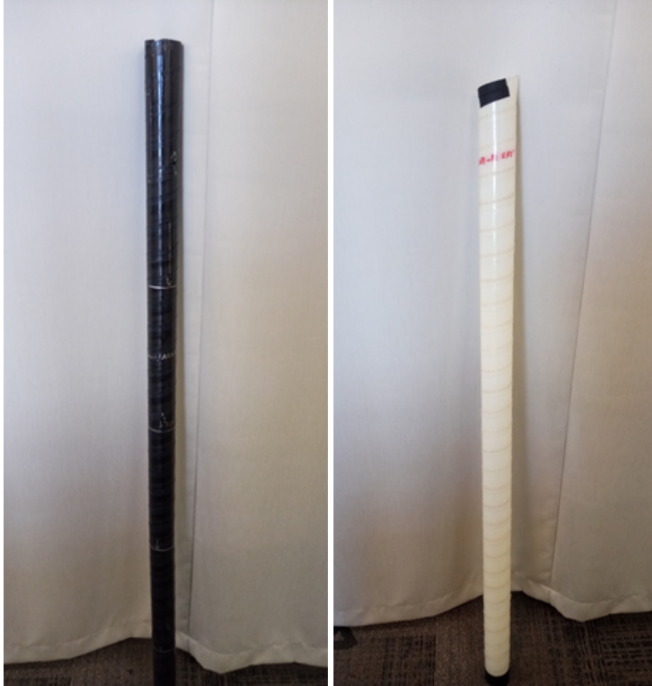
Figure 2.18: Left: the previous ABS band. Right: The new nylon band.
