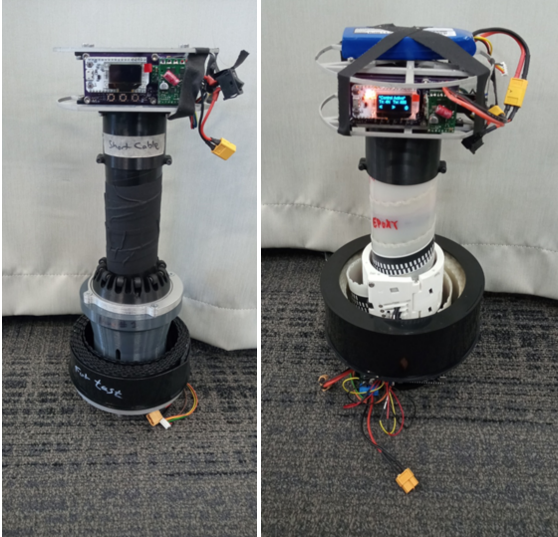
Figure 2.2: The updated edge module core. It uses the same tension cable design, but the band and friction drive have been updated.
