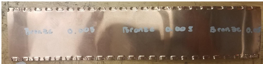
Figure 2.8: A section of 0.005" bronze formed with the ABS dies
