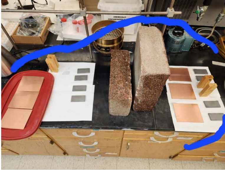
Test Specimens for ASTM B117 Exposure in CSU Q-Fog CCT 1100
