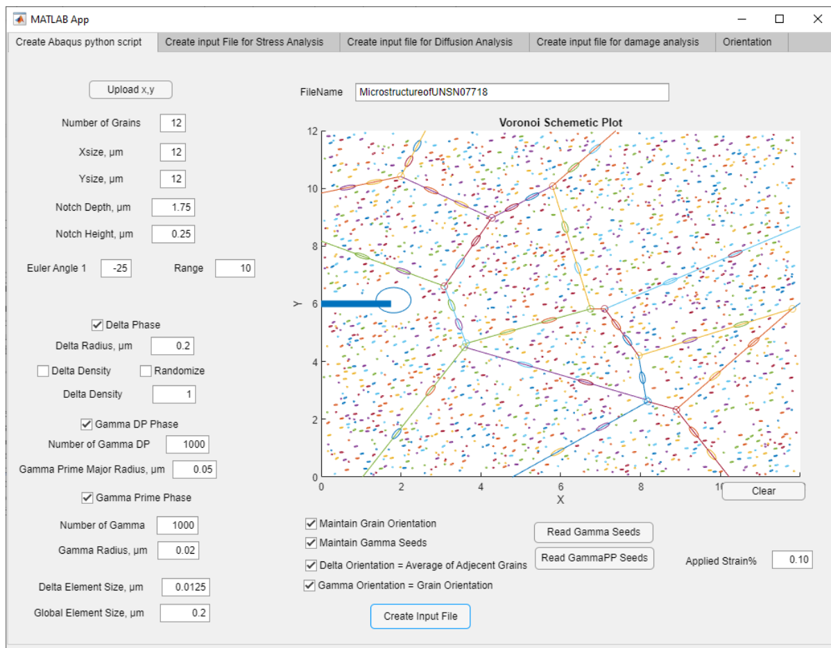
Figure 52 – UI developed to create 2D representative microstructures of Ni-Cr-Mo alloy systems.
