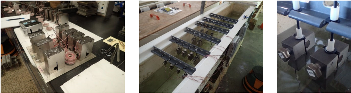
Figure 43 – Instrumented samples showing polysulfide coating protecting the strain gauge for long term exposure. Example photographs of the dry and wet cycle showing the maximum water reached the precrack.
