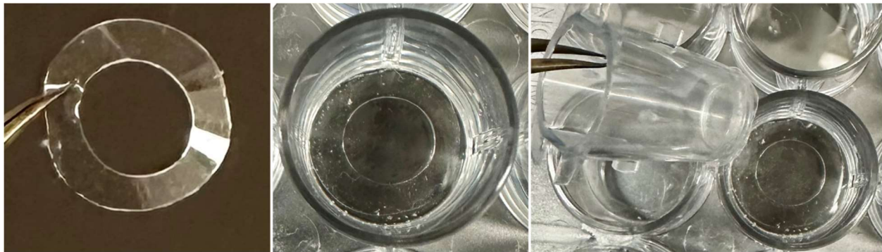
Figure 5. The PDMS inserts for controlled seeding of cells directly below the transwells.
