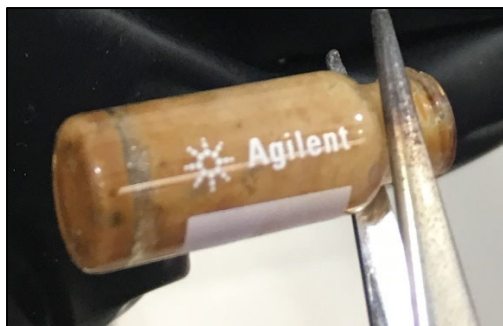
Figure 1. Reaction mixture of HD with \text{Li}_3\text{N} + \text{H}_2\text{O} (22% w/w), sample NB097P143D.
