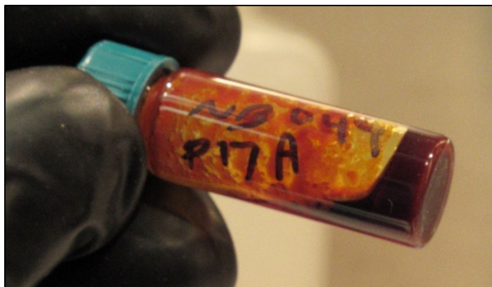
Figure 45. Reaction of HD with [(\text{CH}_3)_2\text{N}]_4\text{Ti} , sample NB0049P17A after two weeks of reaction time.
