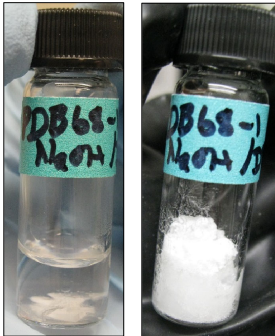
Figure 32. Fully solidified DPCP after four days exposure to a deliquescent slurry of NaOH flakes.
