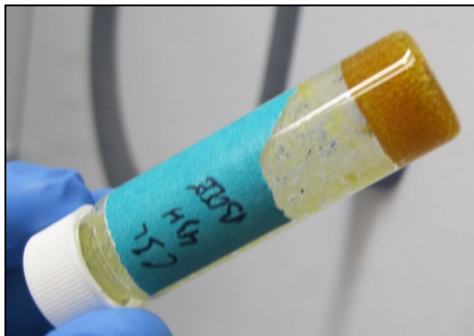
Figure 8. Gelled BCEE/ \text{Li}_3\text{N} /py/MeOH reaction after reacting overnight. Typical LiOH reaction products (grey/white powder) did not form.
