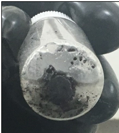
Figure 36. 4.0 mL of HD with pellet F09-138C and 0.4 mL H 2 O. The intact pellet can be seen at the bottom of the vial.
