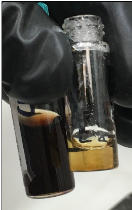
Figure 39. Reaction mixture of HD + LiAlH 4 in THF solution (right, sample nb097P143A), compared to the original HD (left), showing that the reagent removed the color.
