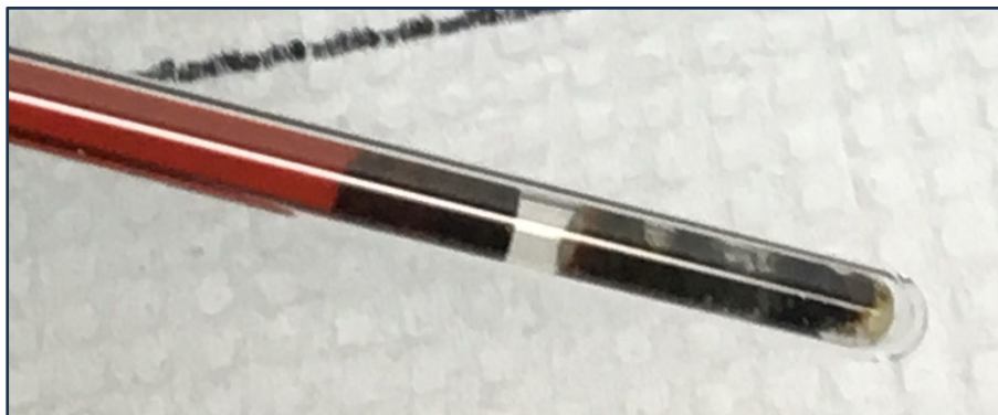
Figure 42. Reaction mixture in NMR tube of HD + MgAl metal + I 2 + DMSO, sample nb097p85A (see Table 2).
