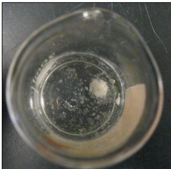
Figure 26. \text{Li}_3\text{N}/\text{Wax} pellet not fully dissolved.
