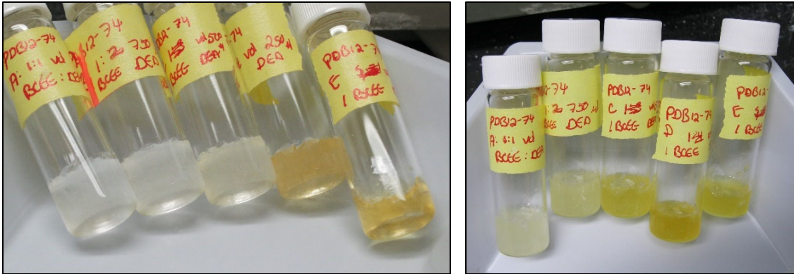
Figure 16. Series of BCEE:DEA mixture ratios after several days; (left) 1 day, (right) 7 days.
