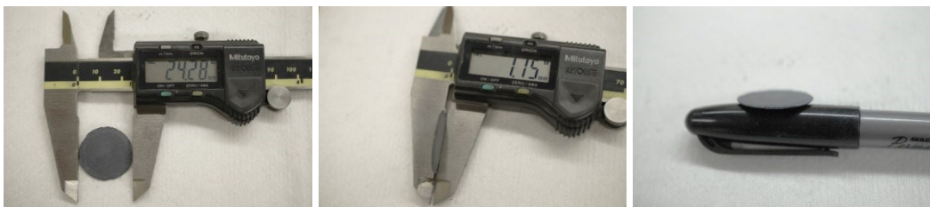
Fig. 8 Well-sintered, dense compact made with synthesized W-KNN powder: (a) diameter, (b) thickness, and (c) relative size, related to a standard Sharpie
