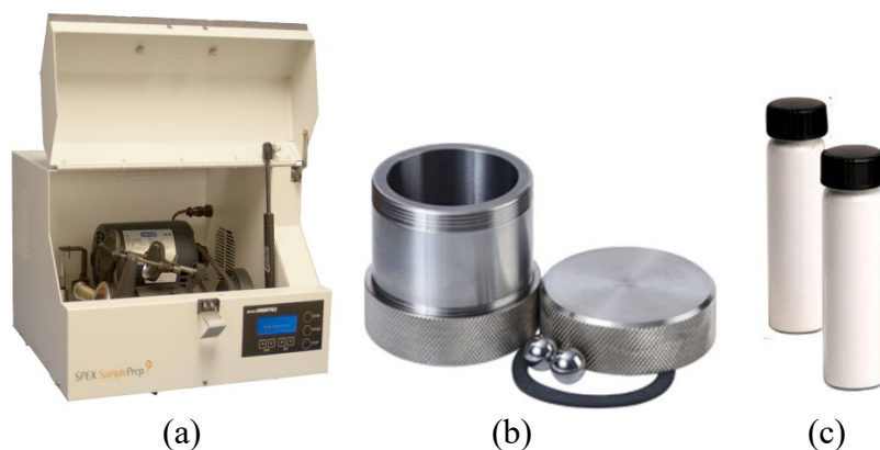
Fig. 1 (a) High-energy ball mill, (b) WC vial and media, and (c) synthesized KNN powder
