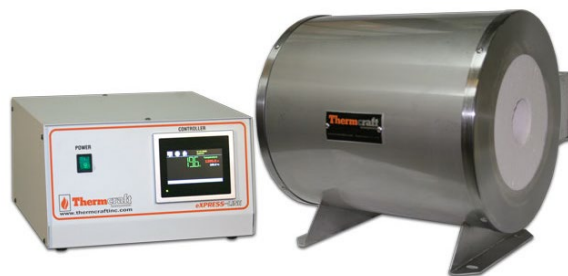
Fig. 3 Thermocraft tube furnace: the milled powder was calcined at 650 °C for 1 h with an Al 2 O 3 tube with the powder placed in an Al 2 O 3 boat
