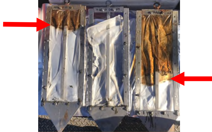
Figure 6. Biofouling lines are marked by red arrows and delineate the sediment – surface water interface.
